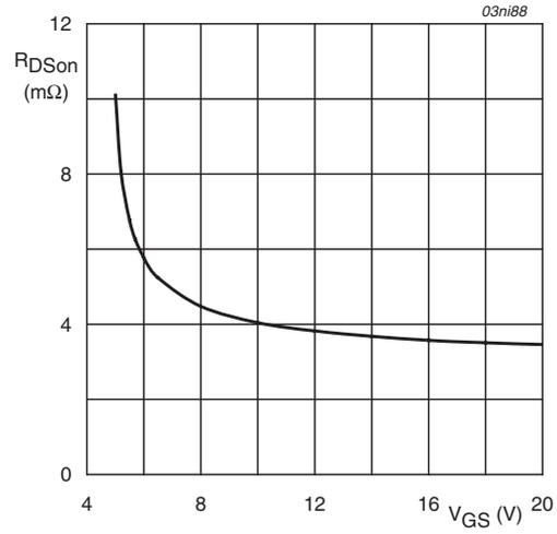
$T_j = 25^\circ\text{C}; I_D = 50\text{A}$
