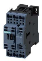
Traction contactor, AC-3 32 A, 15 kW / 400 V 1 NO + 1 NC with solid-state operating mechanism 110 V DC, 0.7-1.25\*Us with integrated varistor 3-pole, size S0 Spring-type terminals
