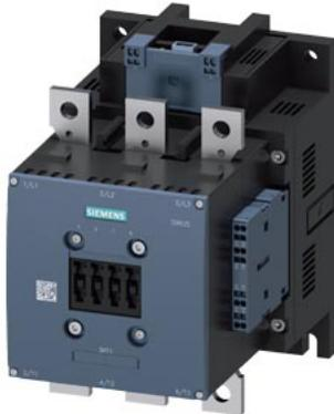
power contactor, AC-3 225 A, 110 kW / 400 V AC (50-60 Hz) / DC operation 21-27 AC/DC, 3 V auxiliary contacts 2 NO + 2 NC 3-pole, frame size S10 busbar connections drive: electronic with PLC interface 24 V DC spring-loaded terminal
