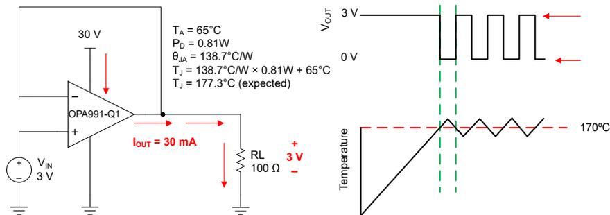
Figure 7-4. Thermal Protection
