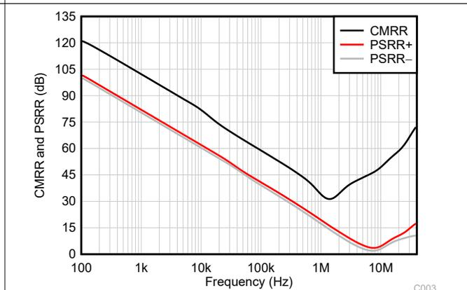
Figure 6-16. CMRR and PSRR vs Frequency
