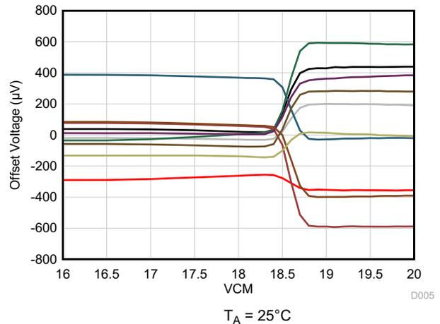
**Figure 6-6. Offset Voltage vs Common-Mode Voltage (Transition Region)**
