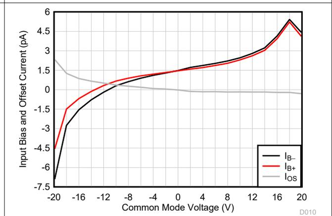
**Figure 6-12. Input Bias Current vs Common-Mode Voltage**
