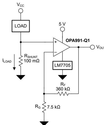
Figure 8-1. OPAx991-Q1 in a Low-Side, Current-Sensing Application
