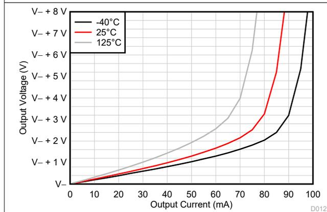
Figure 6-15. Output Voltage Swing vs Output Current (Sinking)
