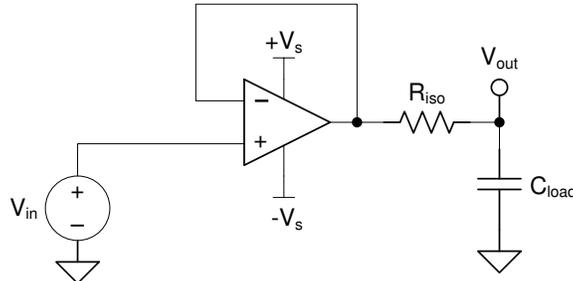
**Figure 7-7. Extending Capacitive Load Drive With the OPAx991-Q1**
