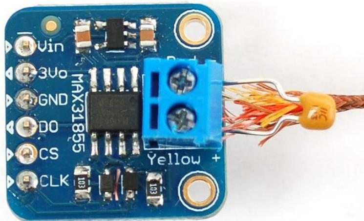
If you are using the MAX31855 v1.0 in a noisy environment, you may need to add a 0.01uF capacitor across the thermocouple leads.
