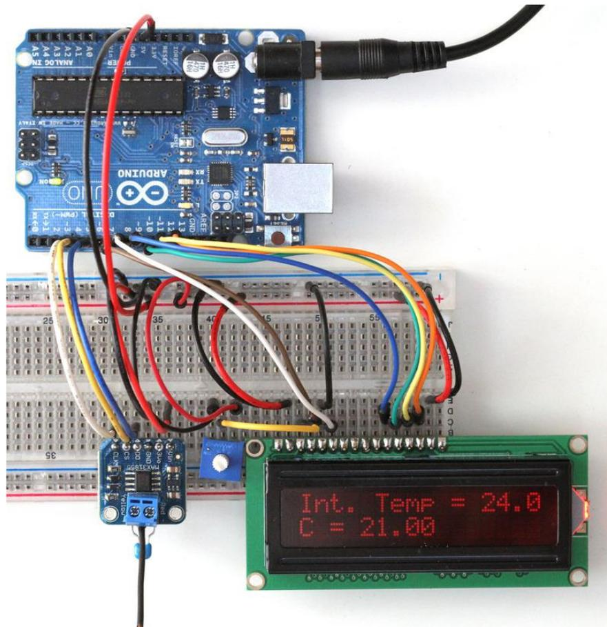
For this wiring, we connected CLK to digital 3, CS to digital 4 and DO to digital 5. Once you get it working, you can change the pin connections in the sketch
