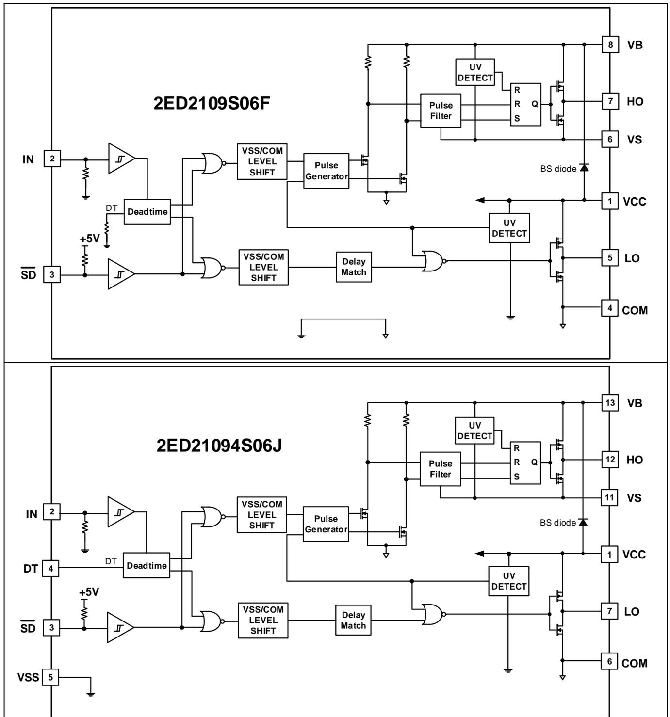
Figure 2 Block diagrams
