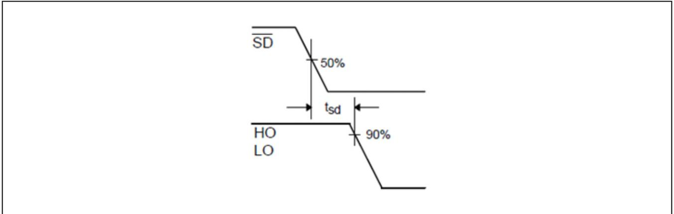
**Figure 12 Shutdown waveform definitions**
