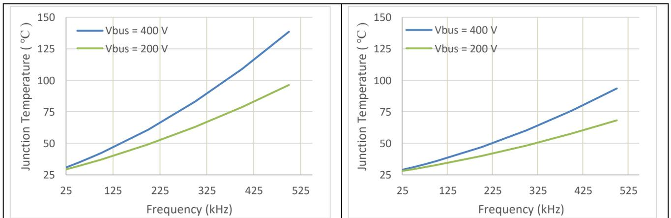
\*Assumptions for above curves: LLC topology, Power switch = IPP60R600P6,  $T_a = 25\text{ }^\circ\text{C}$ ,  $V_{BUS} = 400\text{ V}$ ,  $V_{CC} = 12\text{ V}$ ,  $R_{gon} = 3.9\ \Omega$ ,  $R_{goff} = 1\ \Omega$
