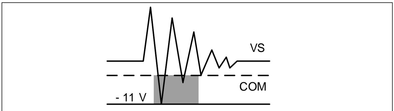
**Figure 23 Headroom for HV level shifter data transmission**
