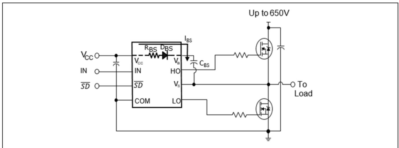
**Figure 17** Half bridge bootstrap circuit in 2ED210x
