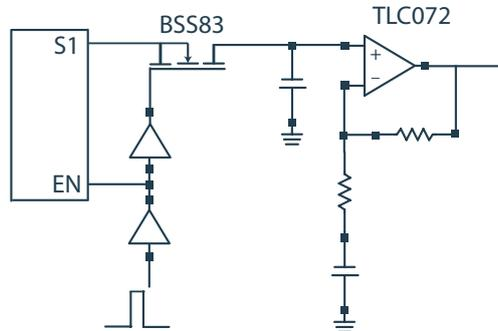
Fig 8: pulsed radar sensor with sample & hold circuitry
