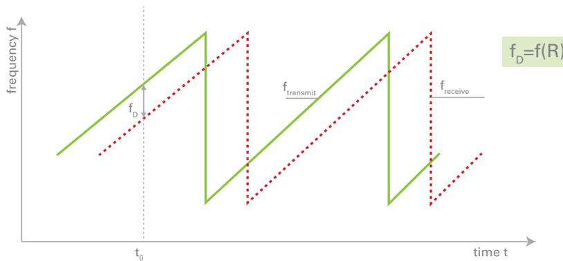
The **FMCW-Radar** for distance measurement only
