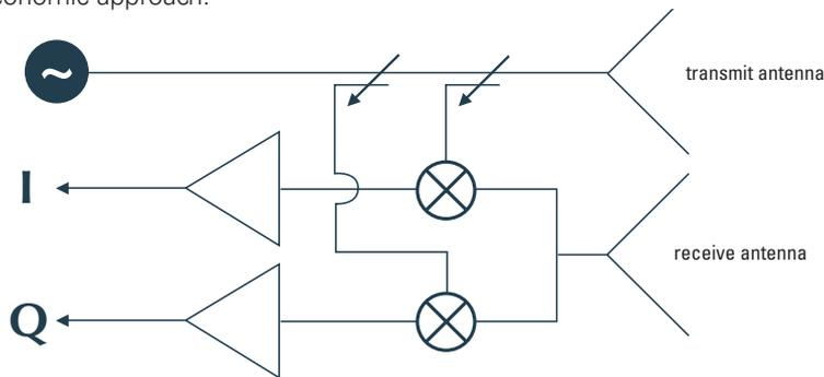
Fig. 5: Schematic of an InnoSenT radar frontend with separate transmit/receive antennas, common transmit/receive antenna as dotted line
