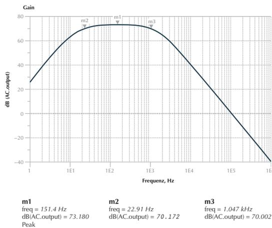
Fig 7: proposal for pre-amplifier circuitry for one channel, 70 dB of gain, 1 kHz bandwidth
