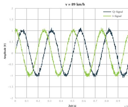
Fig 6: Typical scope shot of the 2 I/Q outputs of a radar sensor from a monotonously moved target
