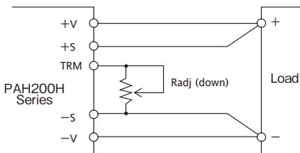
Fig.2-2 Connection for output voltage trim down (1)
