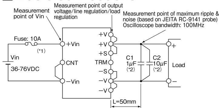
(\*1) 1: The PAH200H series is not equipped with a fuse. Be sure to set a fast-blow fuse for the enhancement of safety and to get approval for safety standards. When using multiple units of the PAH200H series, set a fuse for each unit.
