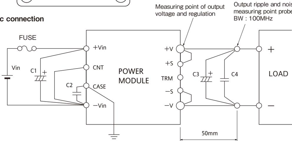
Note : This diagram is for Negative Logic "ON/OFF" Option.
