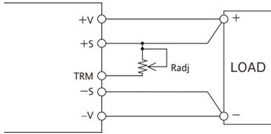
The equation shown below determines the required external resistor ( $R_{adj}$ ) value to obtain a percentage output voltage change of  $\Delta\%$ .
