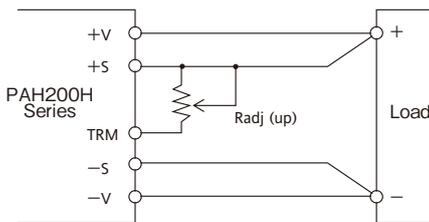
Fig.2-4 Connection for output voltage trim up (2)
