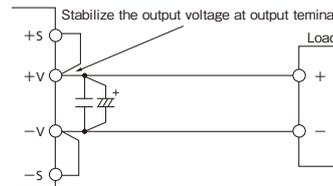
Fig.9-2 Remote Sensing Not in Use (Local Sensing)
