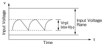
Fig.1-1 Input Ripple Voltage
