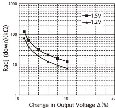
Fig.2-6  $\Delta(\%)$  vs.Radj (down) (3)
