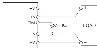
The equation shown below determines the required external resistor (R<sub>adj</sub>) value to obtain a percentage output voltage change of Δ%.
