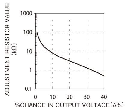
If the external resistor (R<sub>adj</sub>) is connected between the TRIM pin and +S pin, the output voltage will increase. Diagram shown below is the output voltage trim up connection.
