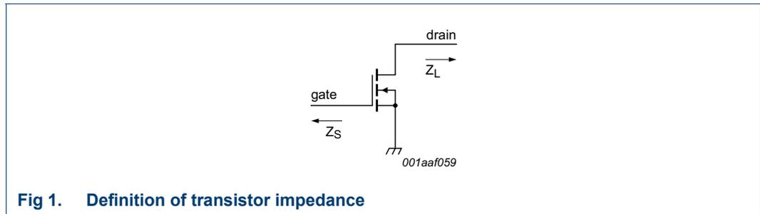
**Fig 1. Definition of transistor impedance**
