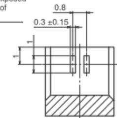
Cross section view A-A (Detector side)
