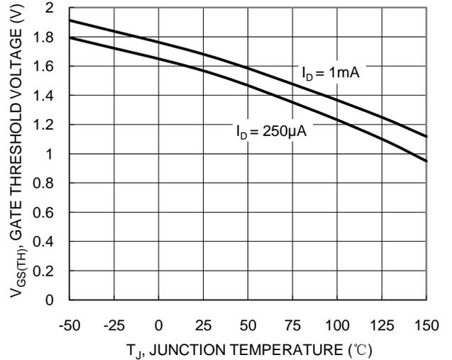
Figure 8. Gate Threshold Variation vs. Junction Temperature
