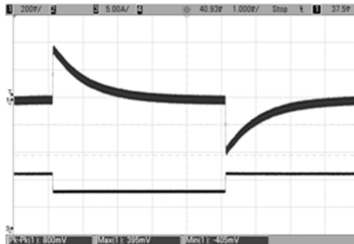
Step Load Transient Response (Vin = 48V, Vout = nom, Cload = 1µF || 10µF, Iout = 50 to 75 to 50% of full load, Ta = +25°C) Ch1 = Vout, Ch2 = Iout.
