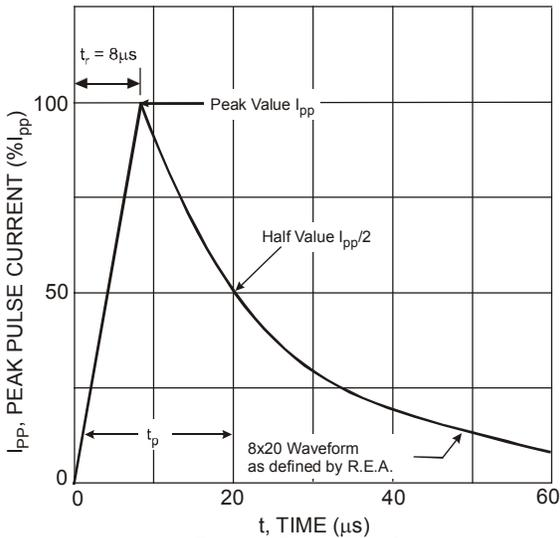
Figure 3 Pulse Waveform
