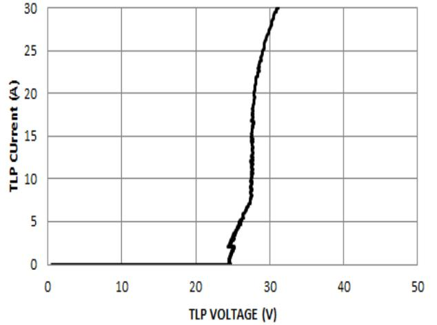
Figure 8 Transmission Line Pulsing (TLP) Current vs. Voltage
