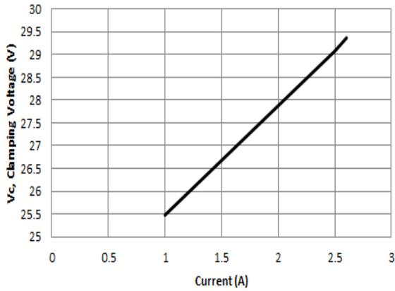
Figure 9 Clamping Voltage Characteristic (tp=8/20uS)
