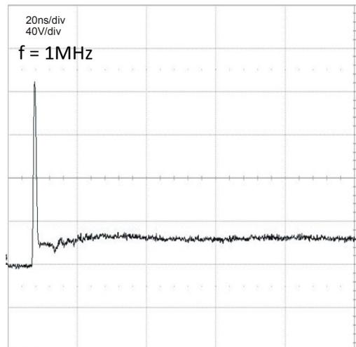
Figure 6 ESD Response to IEC 6100-4-2 (+8kV Contact Discharge)
