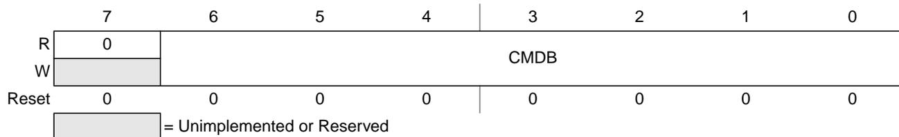
**Figure 2-11. Flash Command Register (FCMD - NVM User Mode)**
