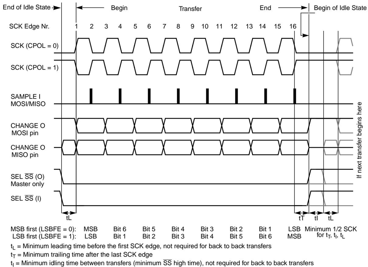
Figure 11-10. SPI Clock Format 1 (CPHA = 1)
