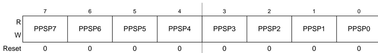
**Figure 4-28. Port P Polarity Select Register (PPSP)**
