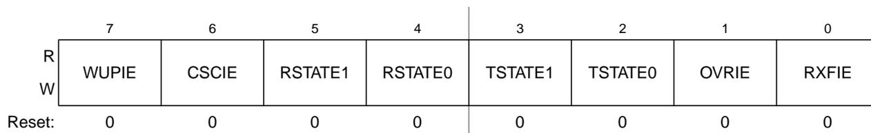
**Figure 9-9. MSCAN Receiver Interrupt Enable Register (CANRIER)**
