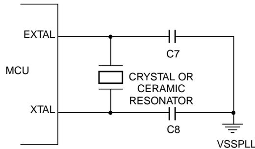
**Figure 1-6. Loop Controlled Pierce Oscillator Connections (PE7 = 1)**
