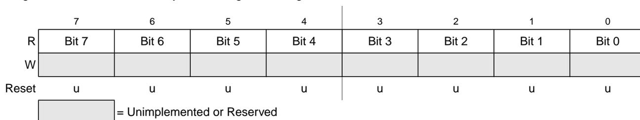
**Figure 16-7. Debug Trace Buffer Register Low (DBGTBL)**
