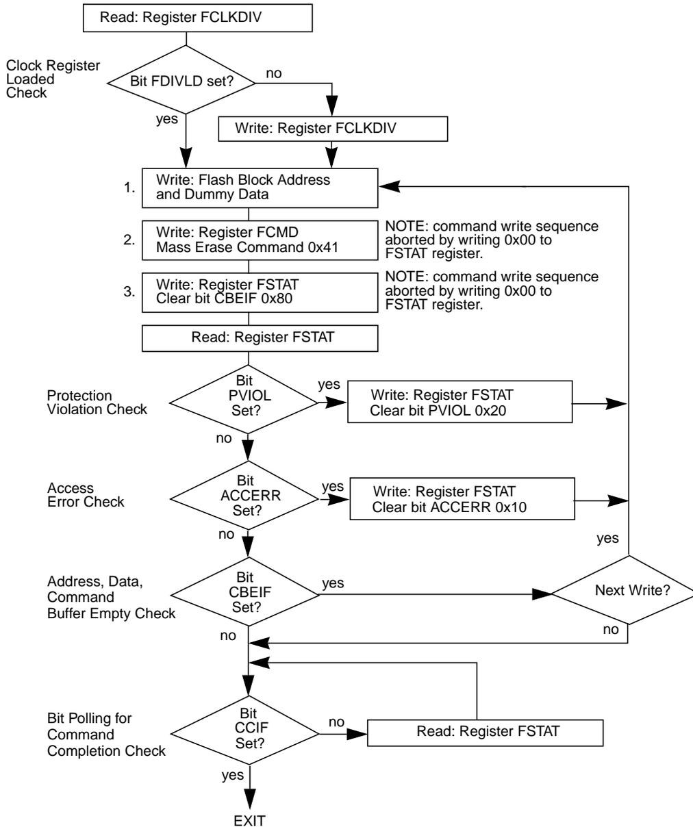
Figure 2-29. Example Mass Erase Command Flow
