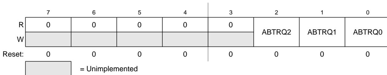
**Figure 9-12. MSCAN Transmitter Message Abort Request Register (CANTARQ)**
