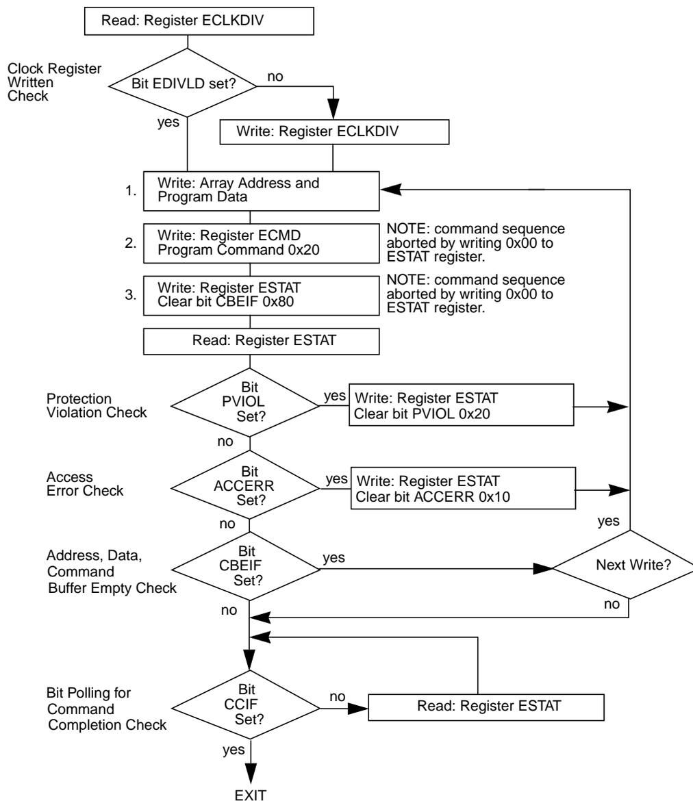
Figure 3-18. Example Program Command Flow
