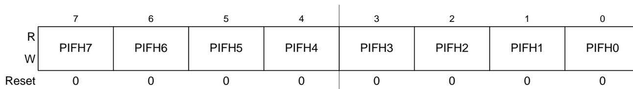
Figure 4-38. Port H Interrupt Flag Register (PIFH)
