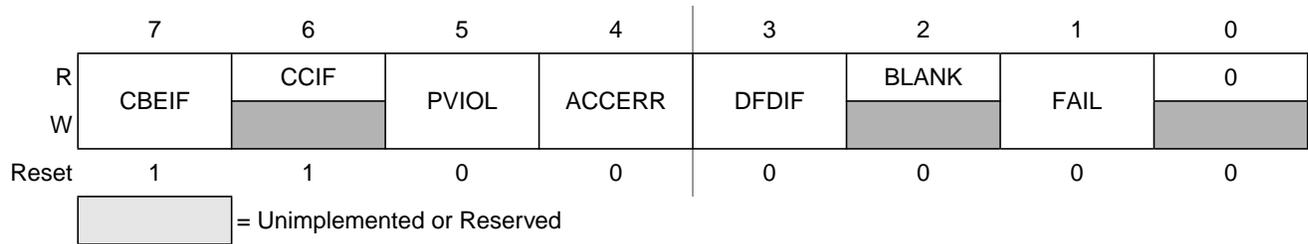
**Figure 2-10. Flash Status Register (FSTAT - Special Mode)**
