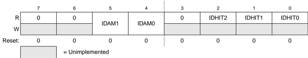
**Figure 9-15. MSCAN Identifier Acceptance Control Register (CANIDAC)**
