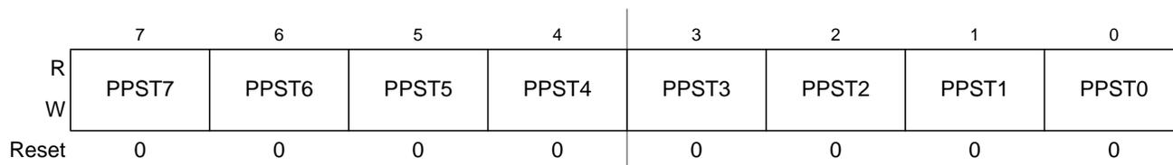
**Figure 4-7. Port T Polarity Select Register (PPST)**
