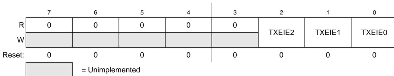
**Figure 9-11. MSCAN Transmitter Interrupt Enable Register (CANTIER)**
