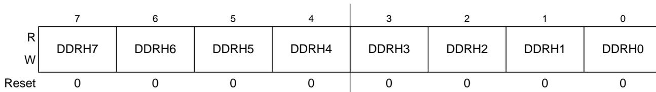
Figure 4-33. Port H Data Direction Register (DDRH)
