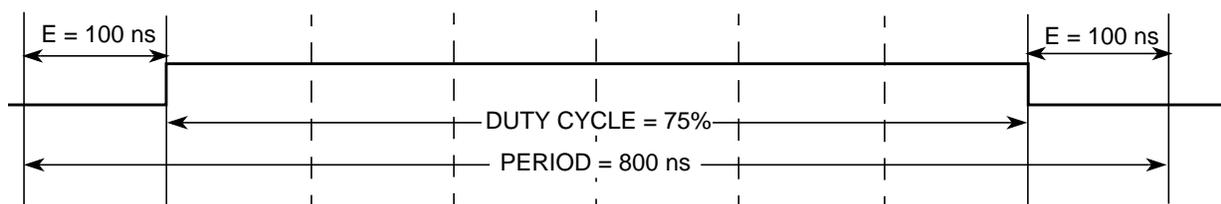
Figure 12-23. PWM Center Aligned Output Example Waveform
