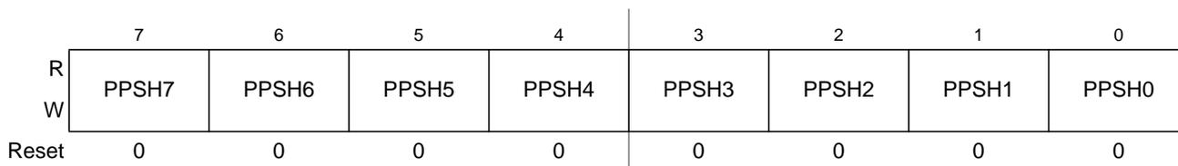
**Figure 4-36. Port H Polarity Select Register (PPSH)**
