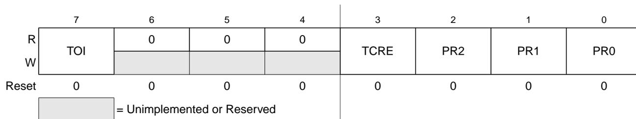
Figure 13-19. Timer System Control Register 2 (TSCR2)
