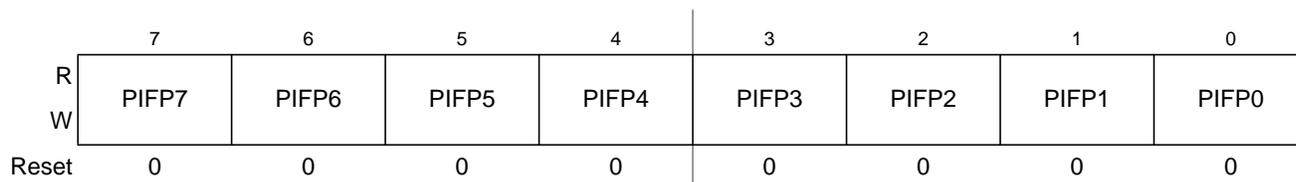
**Figure 4-30. Port P Interrupt Flag Register (PIFP)**
