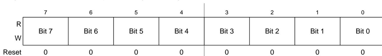
**Figure 16-18. Debug Comparator A Register Low (DBGCAL)**
