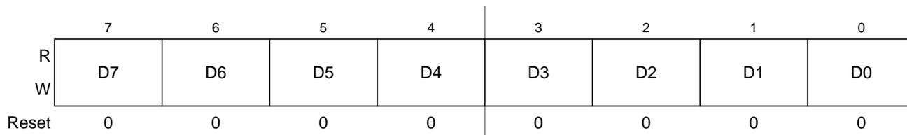
Figure 8-8. IIC Bus Data I/O Register (IBDR)
