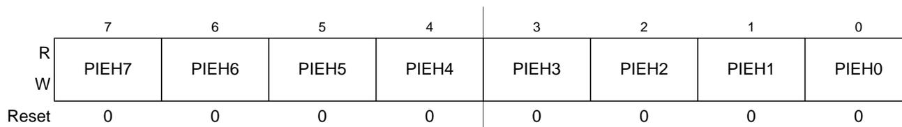
Figure 4-37. Port H Interrupt Enable Register (PIEH)
