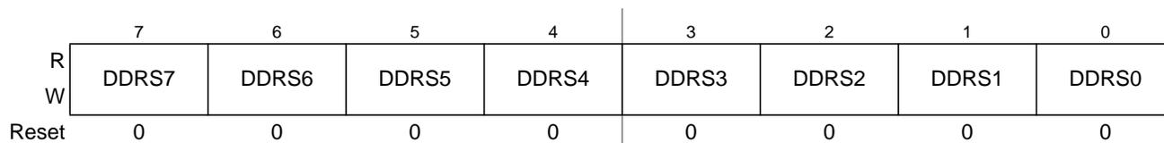
**Figure 4-10. Port S Data Direction Register (DDRS)**
