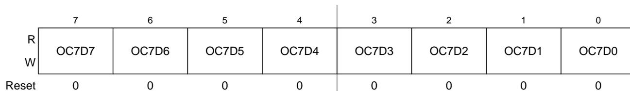
**Figure 13-9. Output Compare 7 Data Register (OC7D)**
