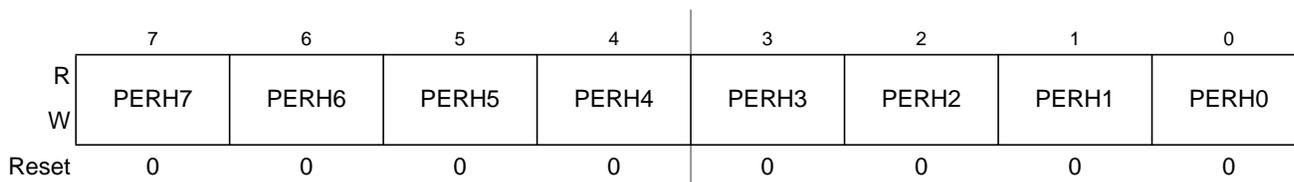
**Figure 4-35. Port H Pull Device Enable Register (PERH)**
