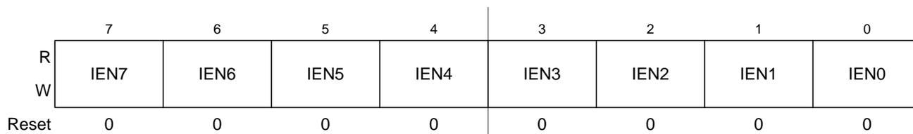
Figure 7-15. ATD Input Enable Register 1 (ATDDIEN1)
