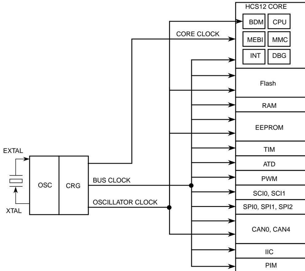
Figure 1-12. Clock Connections
