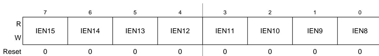
Figure 7-14. ATD Input Enable Register 0 (ATDDIEN0)
