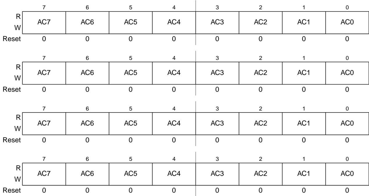
**Figure 9-20. MSCAN Identifier Acceptance Registers (Second Bank) — CANIDAR4–CANIDAR7**
