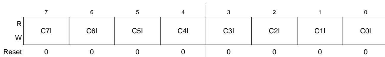
Figure 13-18. Timer Interrupt Enable Register (TIE)
