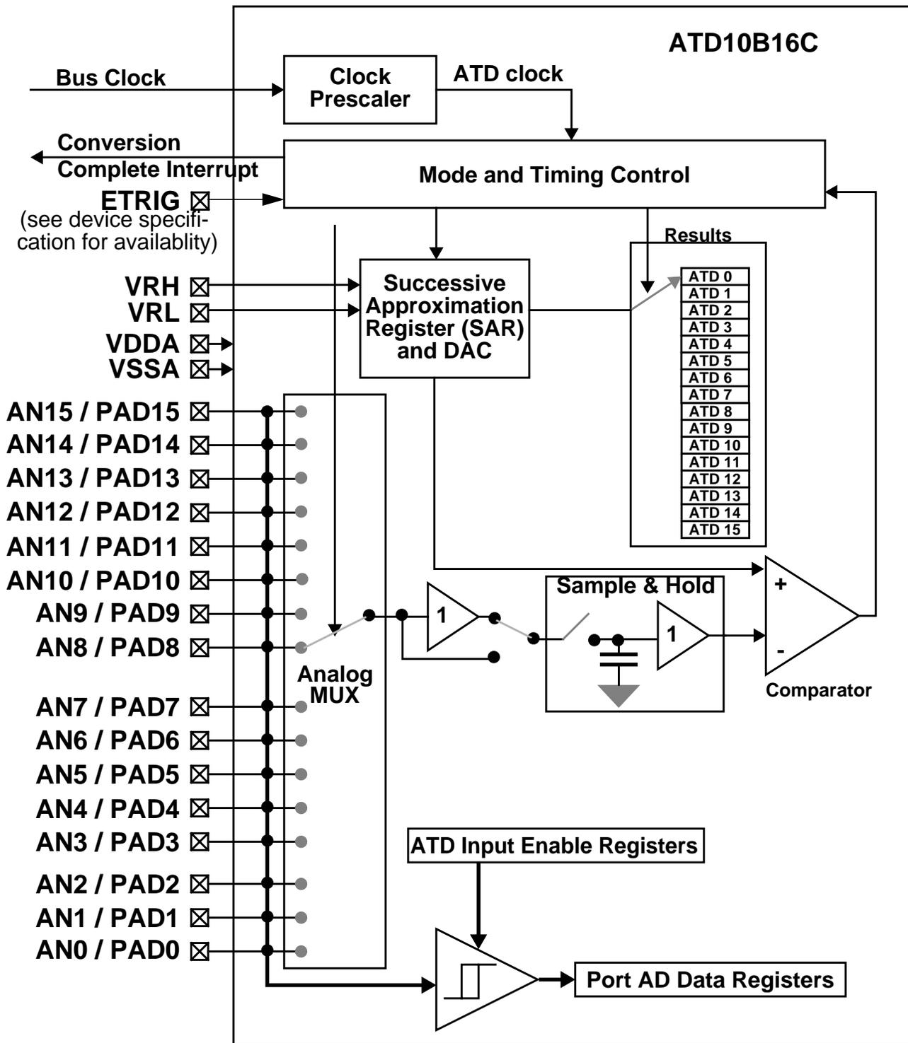
Figure 7-1. ATD10B16C Block Diagram
