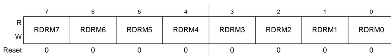
**Figure 4-18. Port M Reduced Drive Register (RDRM)**
