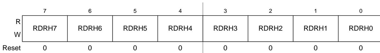
Figure 4-34. Port H Reduced Drive Register (RDRH)
