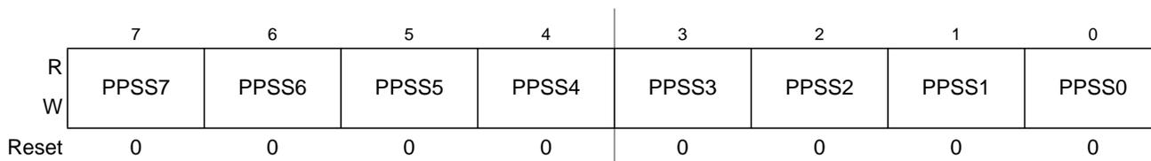
**Figure 4-13. Port S Polarity Select Register (PPSS)**
