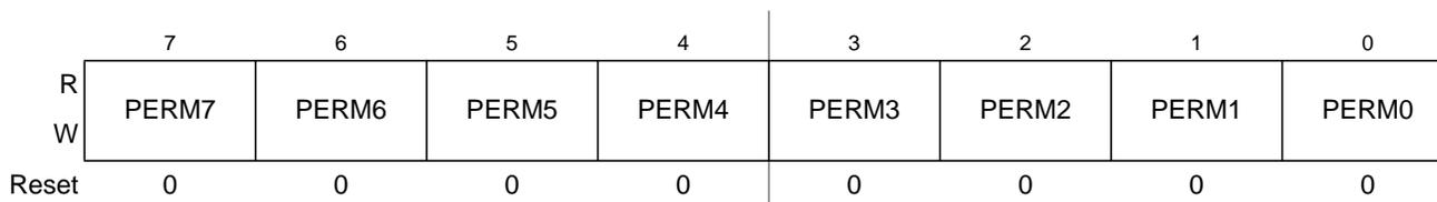
Figure 4-19. Port M Pull Device Enable Register (PERM)
