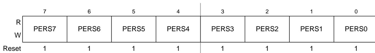
Figure 4-12. Port S Pull Device Enable Register (PERS)
