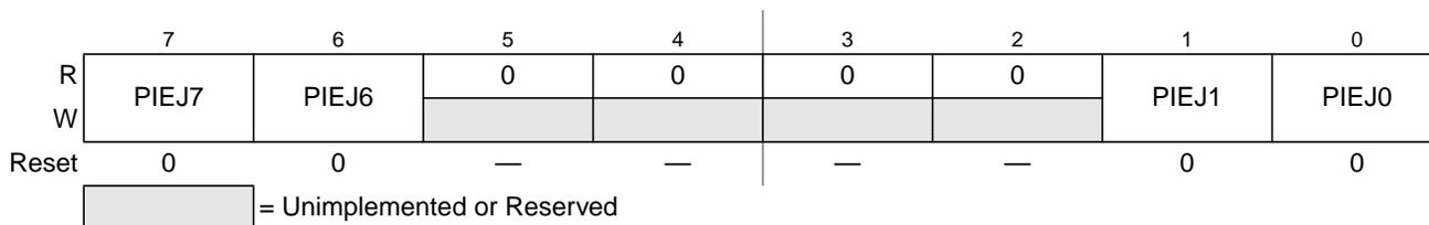
**Figure 4-45. Port J Interrupt Enable Register (PIEJ)**
