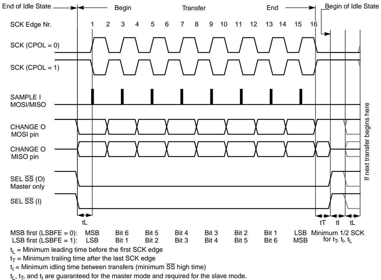
Figure 11-9. SPI Clock Format 0 (CPHA = 0)
