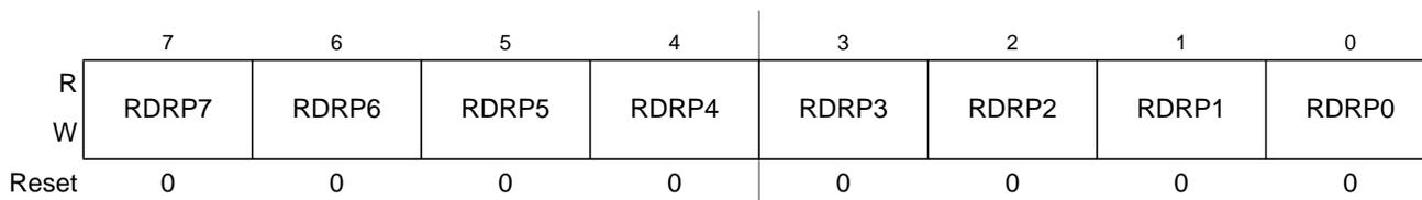
Figure 4-26. Port P Reduced Drive Register (RDRP)
