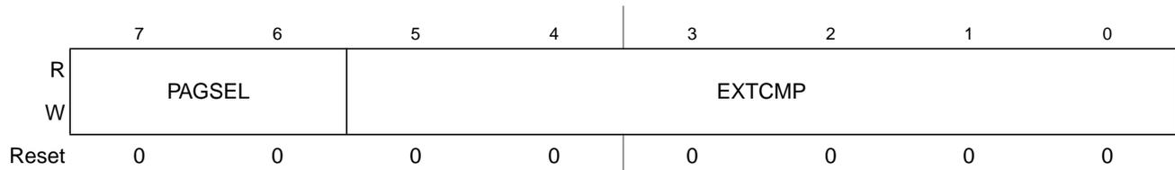
Figure 16-15. Debug Comparator A Extended Register (DBGCAx)
