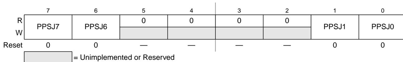
**Figure 4-44. Port J Polarity Select Register (PPSJ)**
