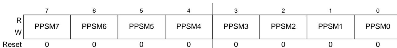
Figure 4-20. Port M Polarity Select Register (PPSM)
