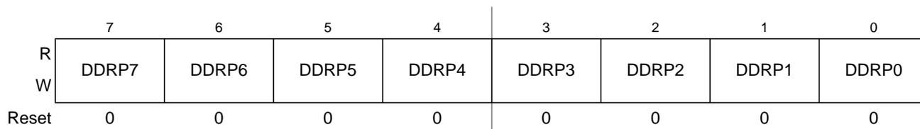
**Figure 4-25. Port P Data Direction Register (DDRP)**
