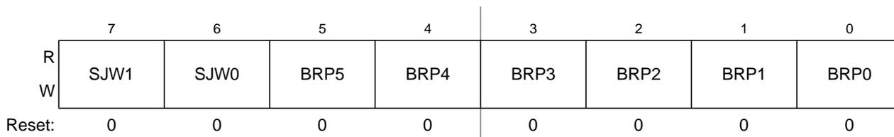
**Figure 9-6. MSCAN Bus Timing Register 0 (CANBTR0)**
