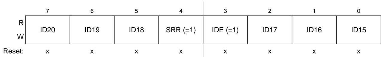
**Figure 9-26. Identifier Register 1 (IDR1) — Extended Identifier Mapping**
