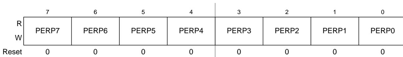
Figure 4-27. Port P Pull Device Enable Register (PERP)
