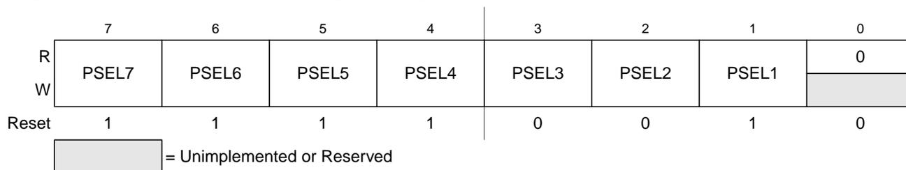
**Figure 17-4. Highest Priority I Interrupt Register (HPRIO)**
