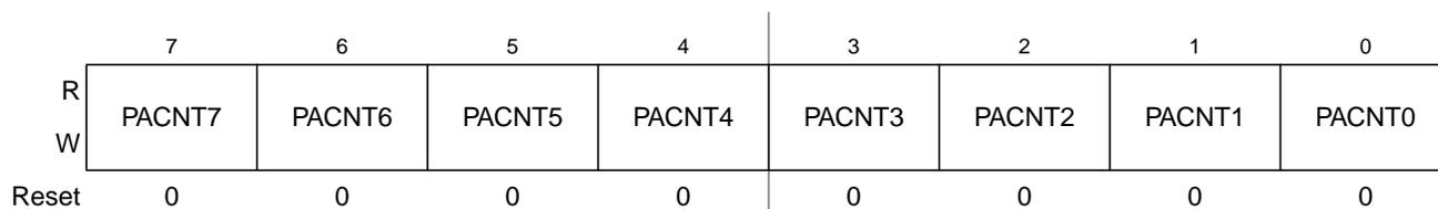
**Figure 13-27. Pulse Accumulator Count Register Low (PACNTL)**
