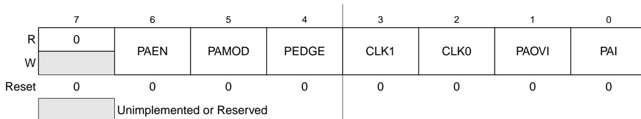
**Figure 13-24. 16-Bit Pulse Accumulator Control Register (PACTL)**
