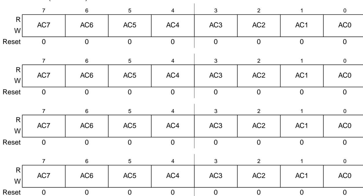
Figure 9-19. MSCAN Identifier Acceptance Registers (First Bank) — CANIDAR0–CANIDAR3
