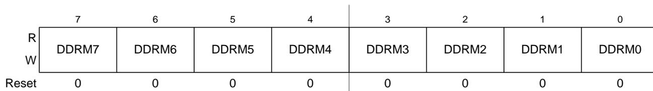
**Figure 4-17. Port M Data Direction Register (DDRM)**
