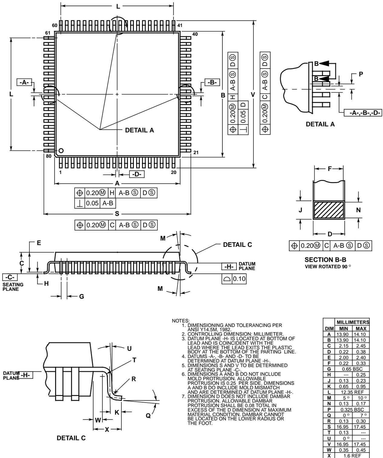
Figure C-2. 80-Pin QFP Mechanical Dimensions (Case no. 841B)
