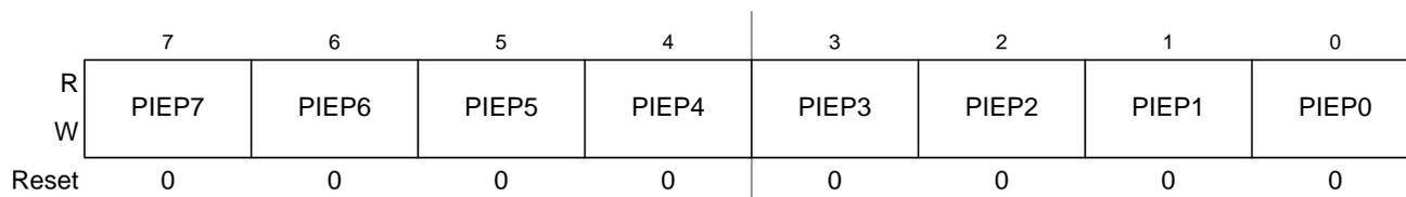
**Figure 4-29. Port P Interrupt Enable Register (PIEP)**
