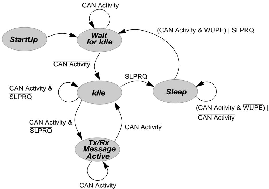
Figure 9-45. Simplified State Transitions for Entering/Leaving Sleep Mode
