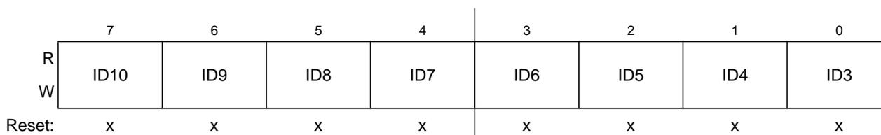
Figure 9-29. Identifier Register 0 — Standard Mapping
