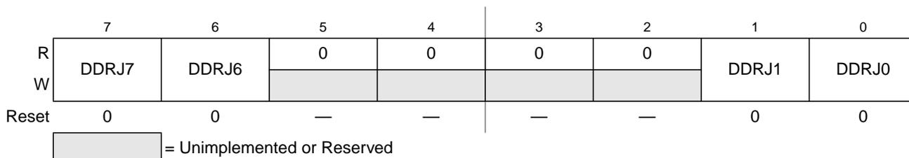
**Figure 4-41. Port J Data Direction Register (DDRJ)**
