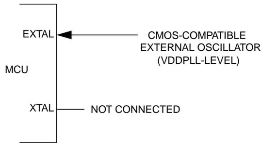
Figure 1-8. External Clock Connections (PE7 = 0)
