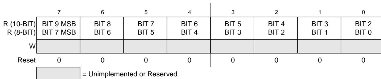
Figure 7-18. Left Justified, ATD Conversion Result Register x, High Byte (ATDDR<sub>x</sub>H)
