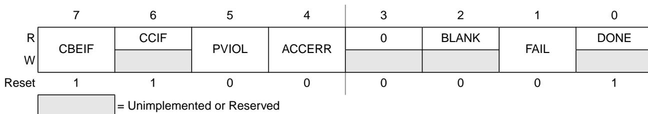
**Figure 3-10. EEPROM Status Register (ESTAT - Special Mode)**
