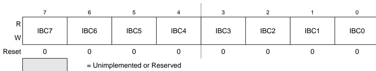
**Figure 8-4. IIC Bus Frequency Divider Register (IBFD)**
