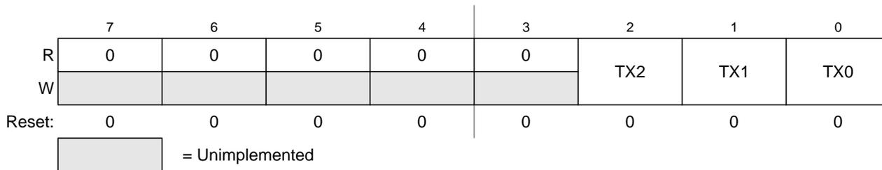
**Figure 9-14. MSCAN Transmit Buffer Selection Register (CANTBSEL)**
