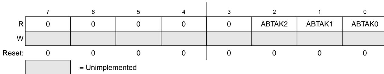
**Figure 9-13. MSCAN Transmitter Message Abort Acknowledge Register (CANTAACK)**
