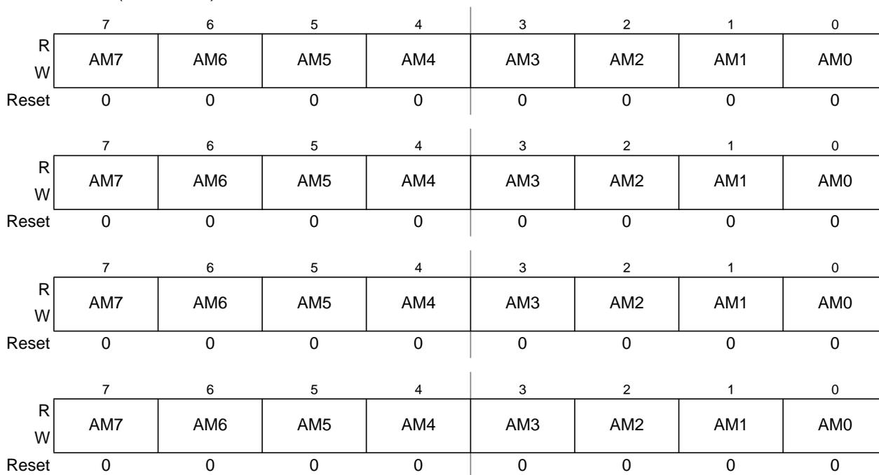
Figure 9-21. MSCAN Identifier Mask Registers (First Bank) — CANIDMR0–CANIDMR3
