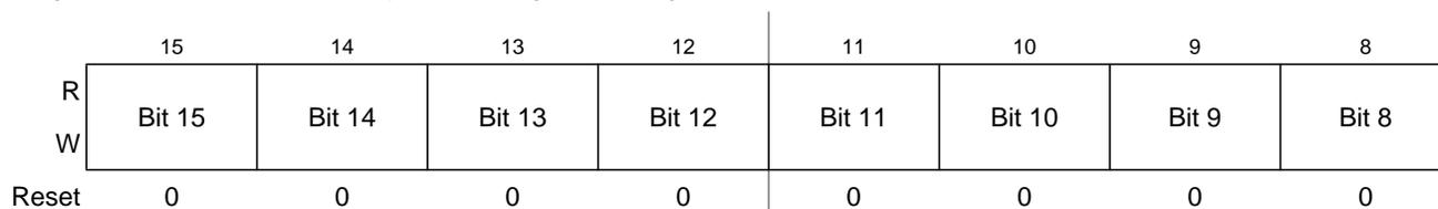
**Figure 16-17. Debug Comparator A Register High (DBGCAH)**
