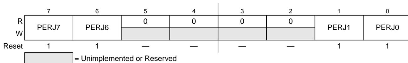
**Figure 4-43. Port J Pull Device Enable Register (PERJ)**
