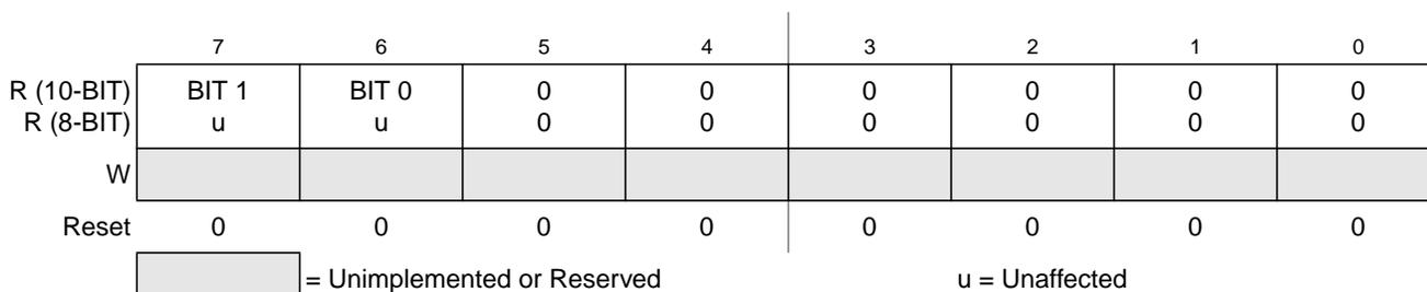
Figure 7-19. Left Justified, ATD Conversion Result Register x, Low Byte (ATDDR<sub>x</sub>L)
