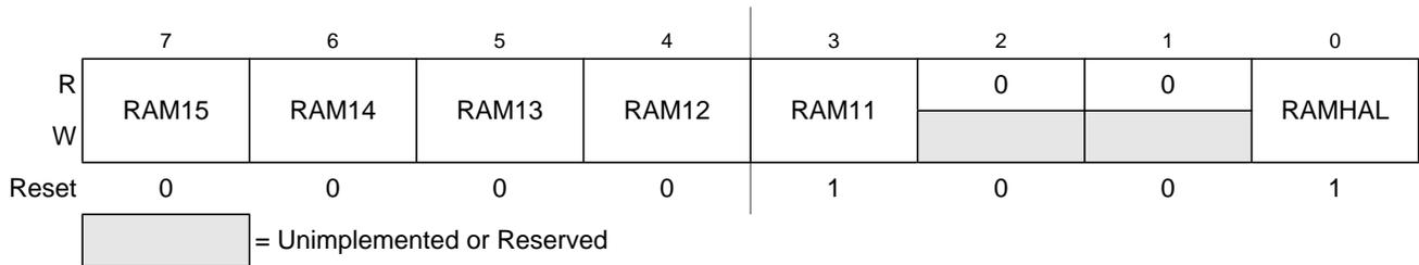
**Figure 19-3. Initialization of Internal RAM Position Register (INITRM)**
