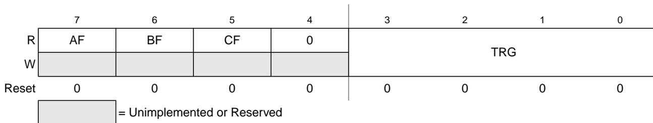
Figure 16-5. Debug Status and Control Register (DBGSC)
