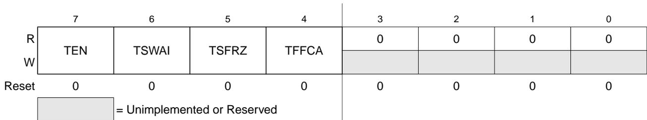
**Figure 13-12. Timer System Control Register 1 (TSCR1)**
