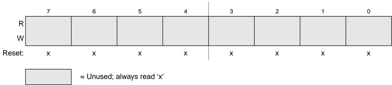
Figure 9-32. Identifier Register 3 — Standard Mapping
