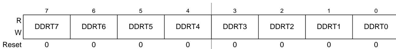
Figure 4-4. Port T Data Direction Register (DDRT)
