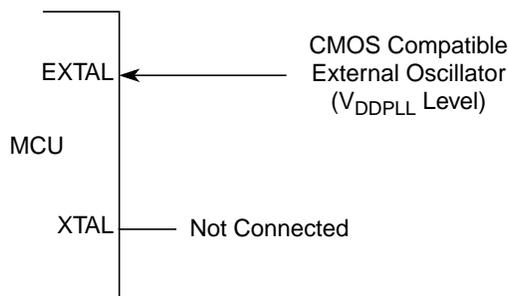
**Figure 6-4. External Clock Connections (XCLKS = 1)**
