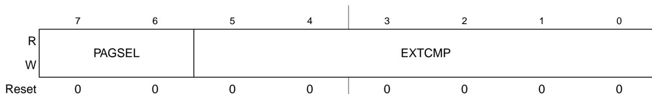
Figure 16-9. Debug Comparator C Extended Register (DBGCCX)
