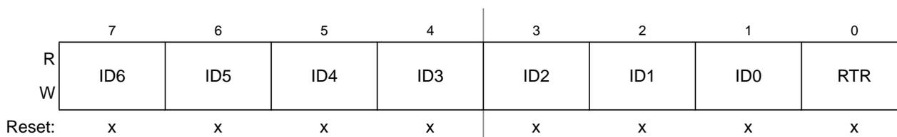
Figure 9-28. Identifier Register 3 (IDR3) — Extended Identifier Mapping
