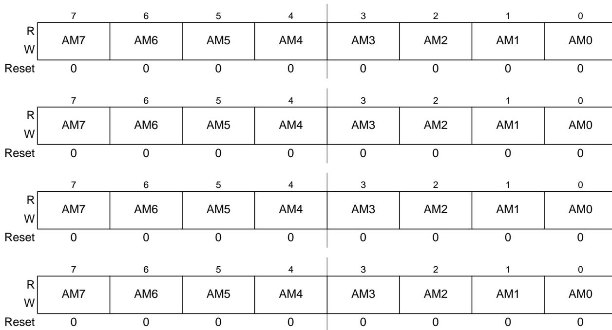
Figure 9-22. MSCAN Identifier Mask Registers (Second Bank) — CANIDMR4–CANIDMR7
