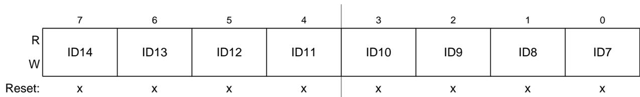
**Figure 9-27. Identifier Register 2 (IDR2) — Extended Identifier Mapping**
