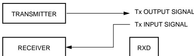
Figure 10-22. Single-Wire Operation (LOOPS = 1, RSRC = 1)
