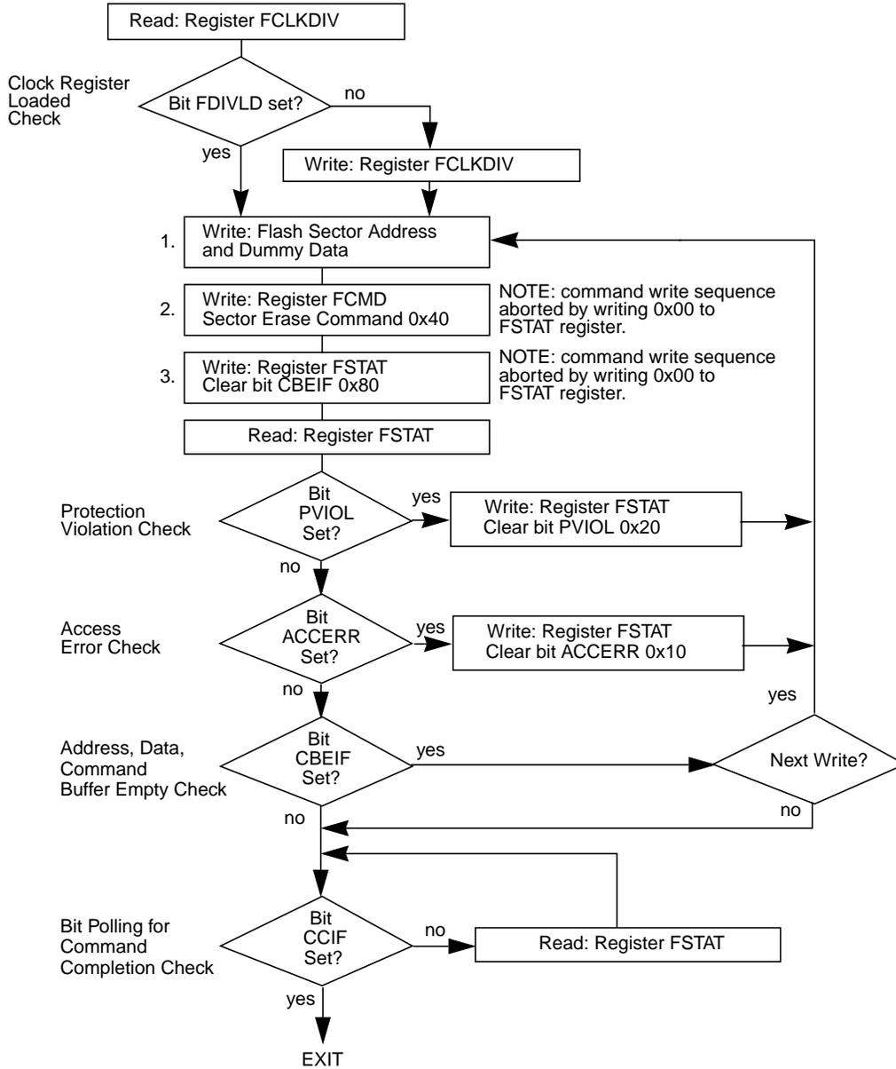
Figure 2-28. Example Sector Erase Command Flow
