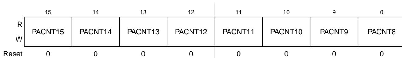
**Figure 13-26. Pulse Accumulator Count Register High (PACNTH)**
