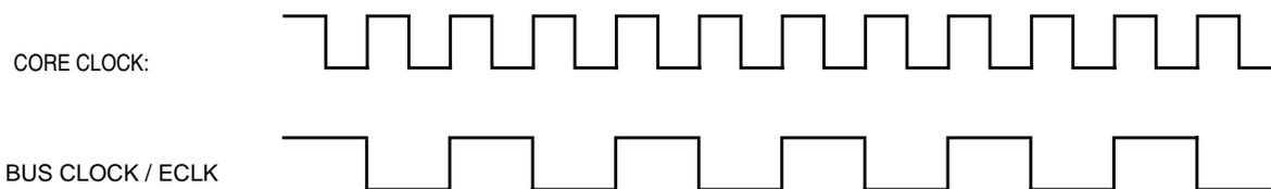
Figure 5-18. Core Clock and Bus Clock Relationship
