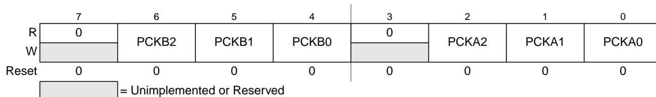
**Figure 12-6. PWM Prescale Clock Select Register (PWMPRCLK)**
