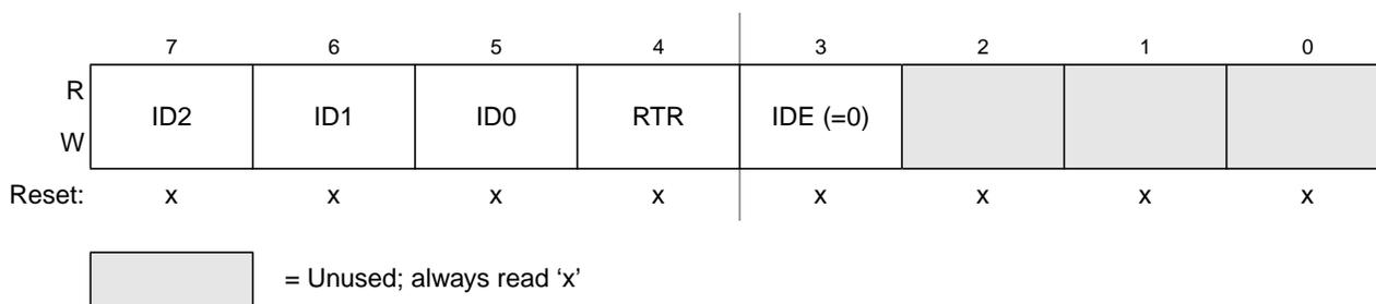
**Figure 9-30. Identifier Register 1 — Standard Mapping**
