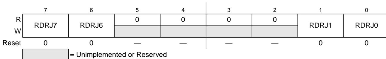
**Figure 4-42. Port J Reduced Drive Register (RDRJ)**
