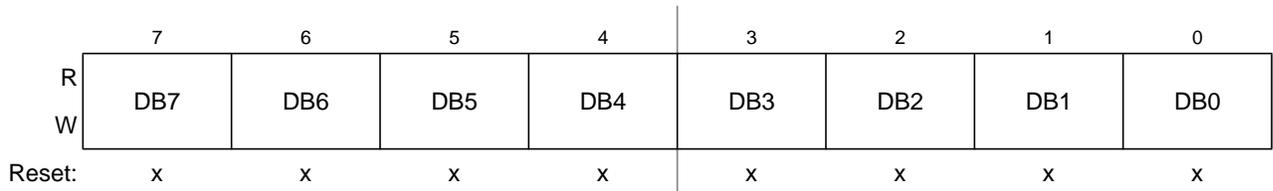
Figure 9-33. Data Segment Registers (DSR0–DSR7) — Extended Identifier Mapping
