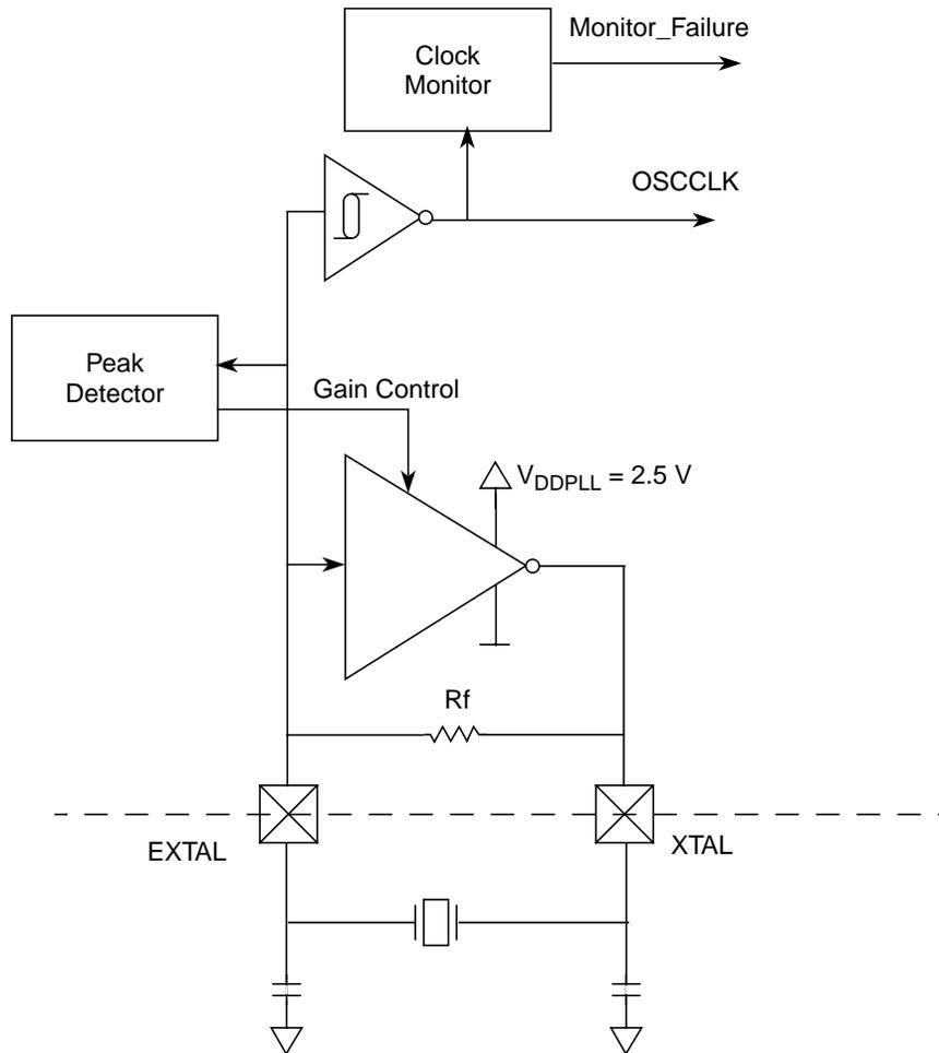
Figure 6-1. XOSC Block Diagram
