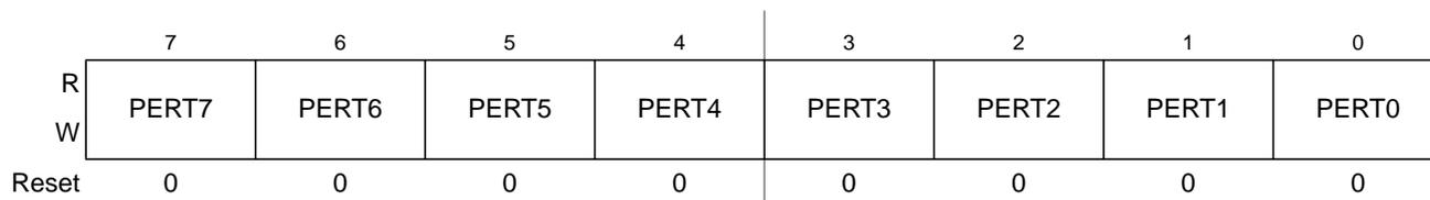
**Figure 4-6. Port T Pull Device Enable Register (PERT)**
