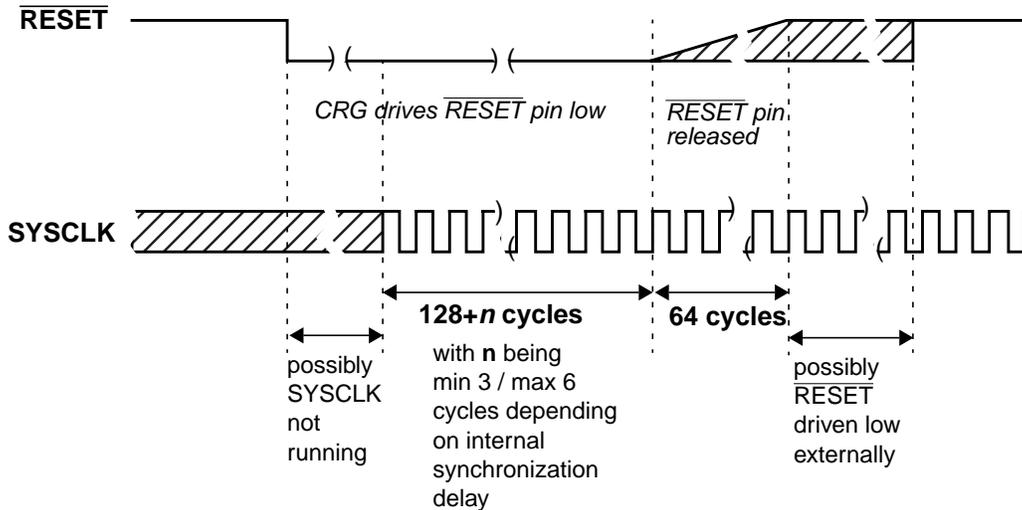
Figure 5-25.  $\overline{\text{RESET}}$  Timing
