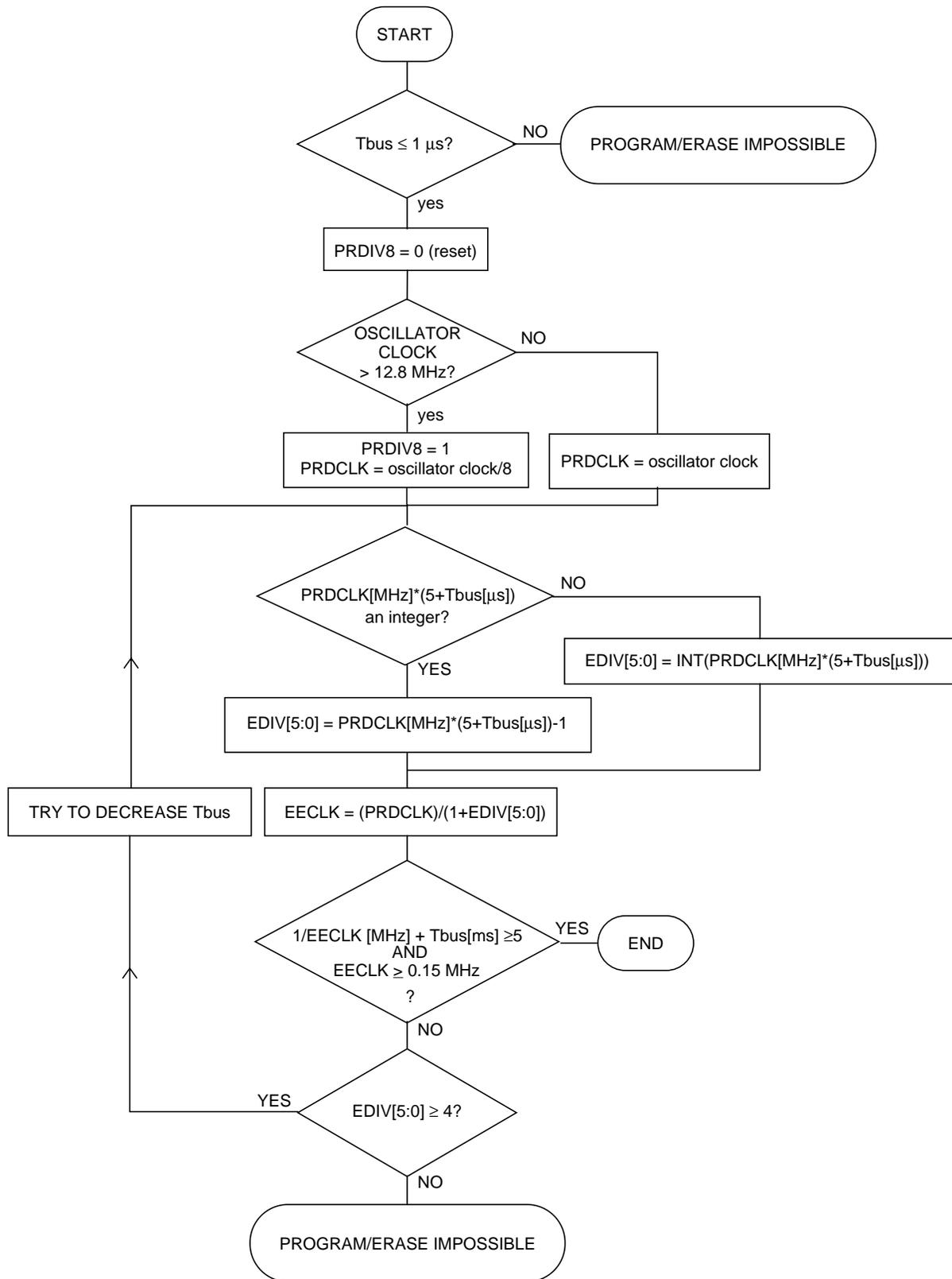
Figure 3-17. PRDIV8 and EDIV Bits Determination Procedure
