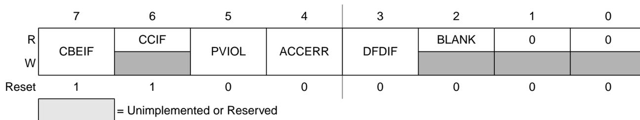
**Figure 2-9. Flash Status Register (FSTAT - Normal Mode)**
