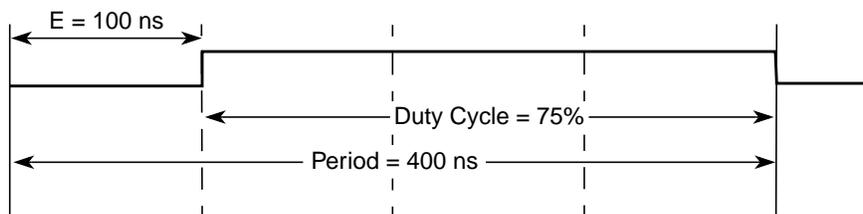
Figure 12-21. PWM Left Aligned Output Example Waveform
