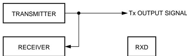
Figure 10-23. Loop Operation (LOOPS = 1, RSRC = 0)
