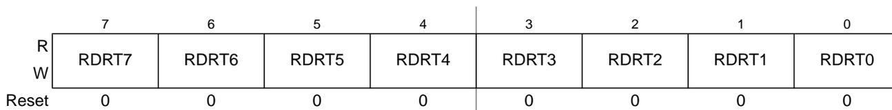
Figure 4-5. Port T Reduced Drive Register (RDRT)
