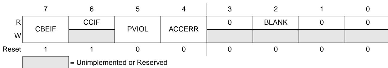
**Figure 3-9. EEPROM Status Register (ESTAT - Normal Mode)**
