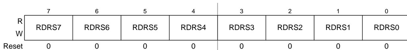
Figure 4-11. Port S Reduced Drive Register (RDRS)
