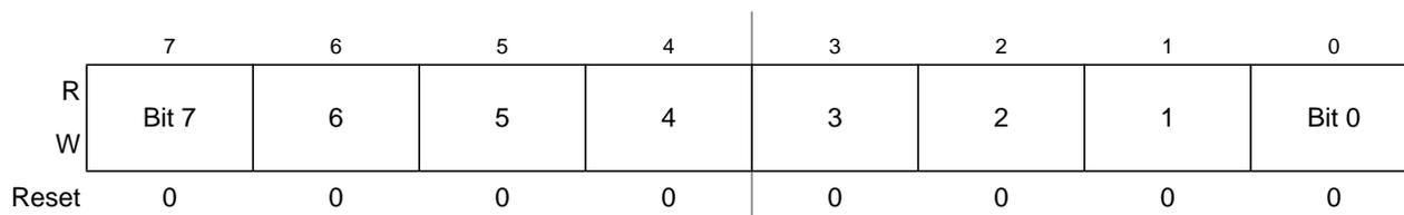
Figure 18-20. Port K Data Direction Register (DDRK)
