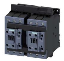
Reversing contactor assembly, AC-3, 30 kW 400 V, 0.7...1.25 US DC, 24 V DC 3-pole, Size S2 screw terminal electrical and mechanical interlock 2 NO integrated Varistor mounted
