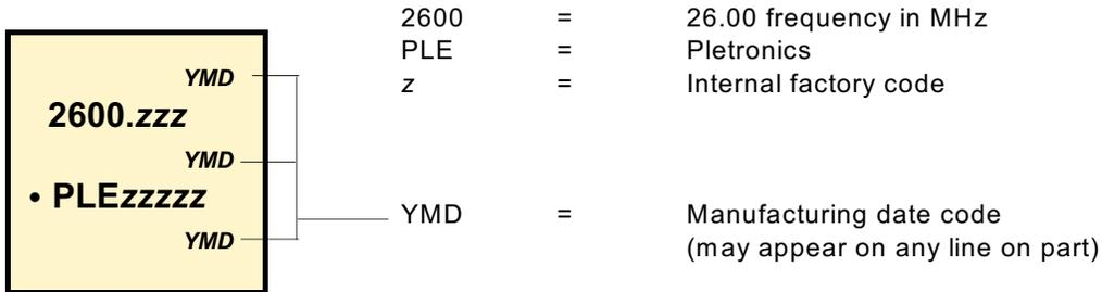
The actual part number is TCD4027-26.0M where the model number "027" is the specification number the part is made to. This is not included in the part marking. This is included on the label on the Tape and Reel.
