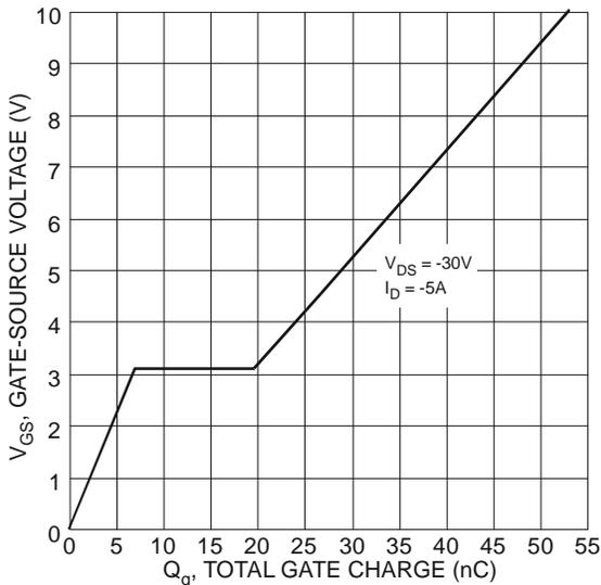
Figure 11 Gate-Charge Characteristics
