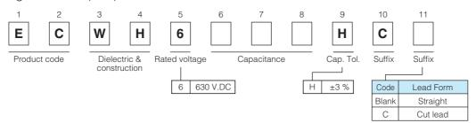
Rated voltage 630 V.DC (Odd size taping)
