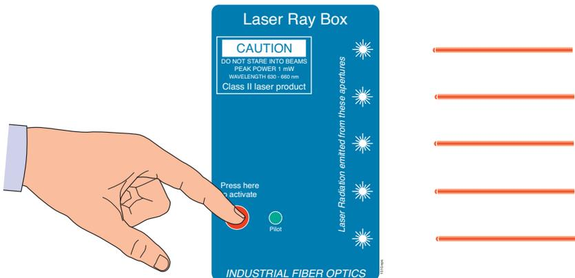
**Figure 6. Laser Ray Box emitting 5 parallel light rays**
