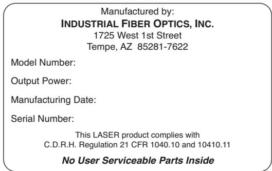
**Figure 3. Laser certification and identification label.**
