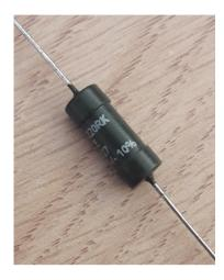
TE Connectivity HPCR Series Axial Leaded Non-Inductive Bulk Ceramic Resistors provide excellent performance where high peak power or high-energy pulses must be handled in a small size. The advantage of the bulk construction is that it produces an inherently noninductive resistor; and it allows energy and power to be uniformly distributed through the entire ceramic resistor body — there is no film or wire to fail.
