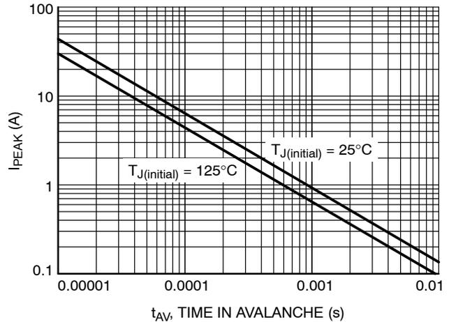
Figure 12. Maximum Drain Current vs. Time in Avalanche
