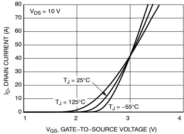
Figure 2. Transfer Characteristics
