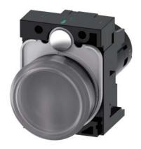
Indicator light with LED lamp, compact, 22 mm, round, plastic, clear with red-yellow-green LED, lens, smooth, with holder, operating voltage 6-24 V AC/DC, screw terminal
