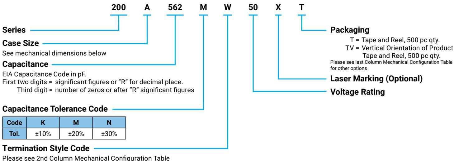
The above part number refers to a 200 A Series (case size A) 5600 pF capacitor, M tolerance (±20%), 50 WVDC, with W termination (Tin / Lead, Solder Plated over Nickel Barrier), Laser Marking and Tape and Reel 1000 pc qty. Packaging
