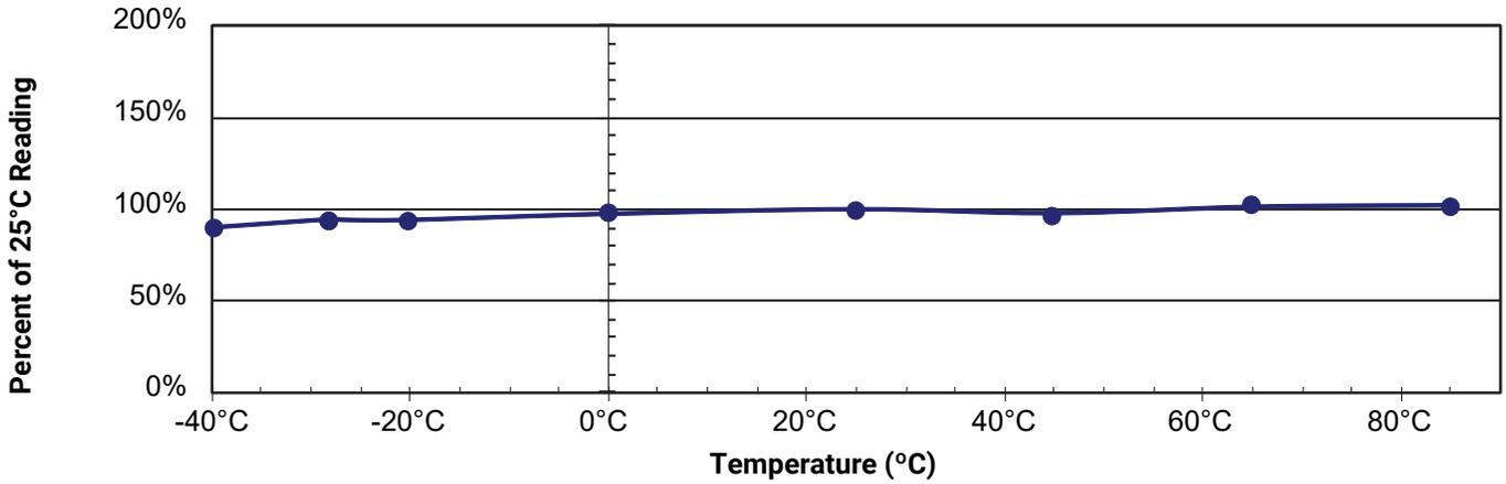
LEAKAGE CURRENT VS. TEMPERATURE
