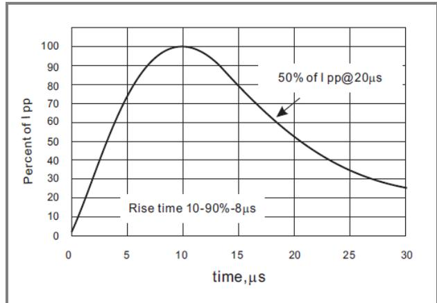
Fig.4 8/20 Pulse Waveform
