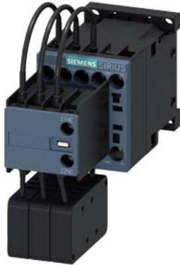
Capacitor contactor, AC-6b 12.5 kVAR, / 400 V 1 NO + 1 NC, 220 V AC, 50 Hz 240 V, 60 Hz 3-pole, Size S00 screw terminal
