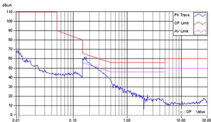
■ **Conduction Testing<sup>[3]</sup> 2 (110Vac/60Hz)**
