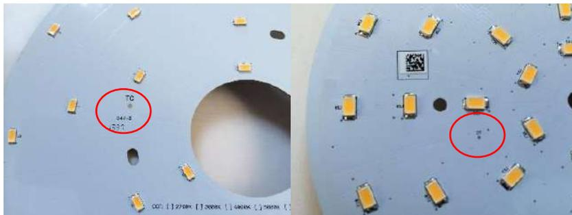
You can use the high-temperature thermal conductivity glue (Such as SatlonD-3/606...etc.) to fix the thermal couple to the  $T_C$  point then measure the temperature. Once you got the  $T_C$  temperature measurement data, you can calculate the junction temperature based on the measurement data of the  $T_C$ . The details of the calculation method are shown in the following page:
