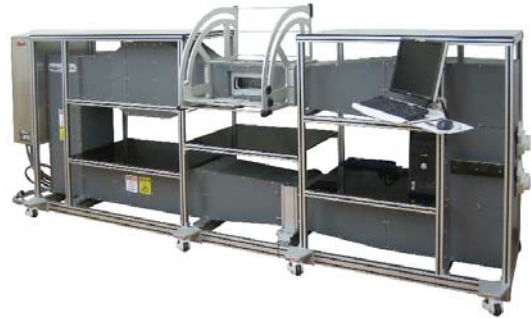
Fig. F: FDK Original Wind Tunnel
