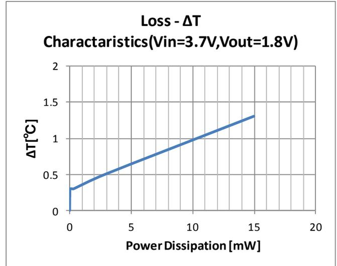
The output current of the device may need to be de-rated if it is operated in a high ambient temperature or in a continuous power delivering application. The amount of current de-rating is highly dependent on the environmental thermal conditions, i.e. PCB design, nearby components or effective air flows. Care should especially be taken in applications where the device temperature exceeds 85°C.
