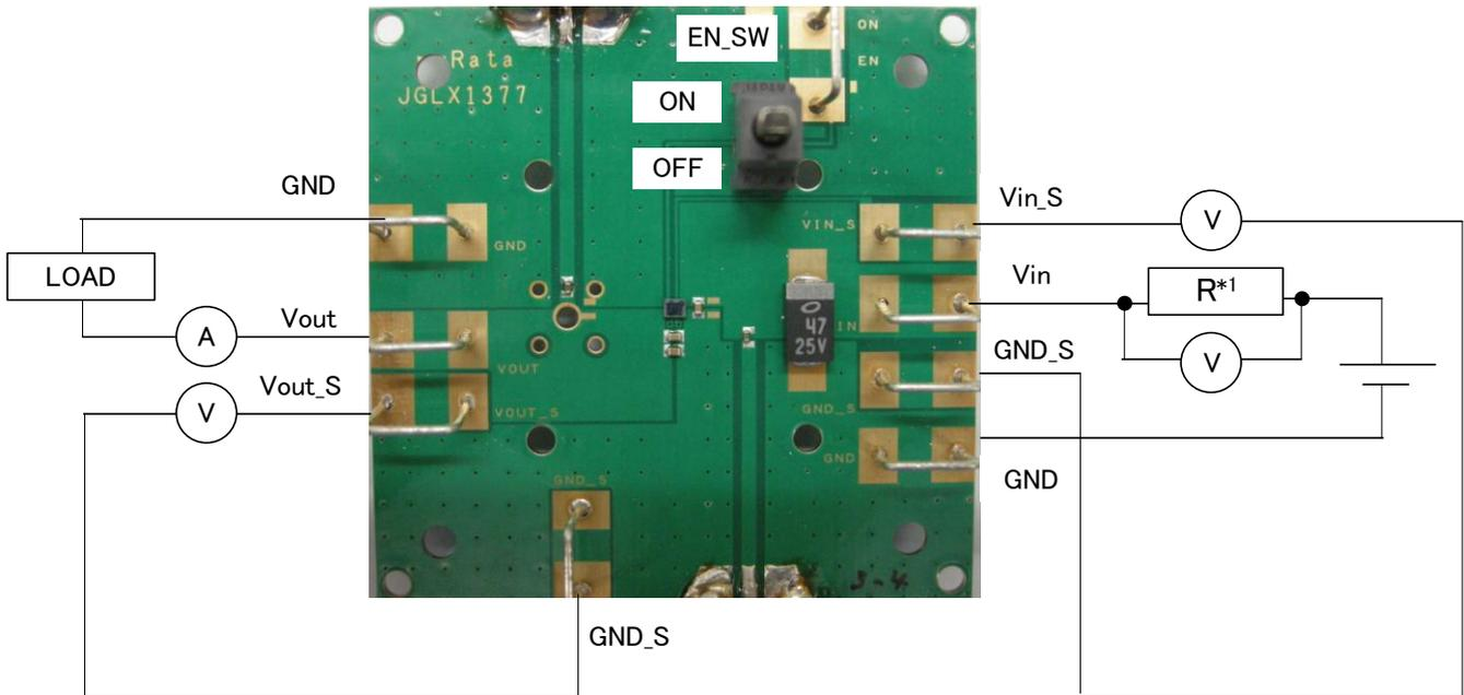
\*1 : Using Resistor (ex : 100Ω) is recommended to measure  $I_{in}$
