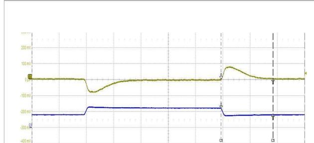
Output voltage response to load current step-
