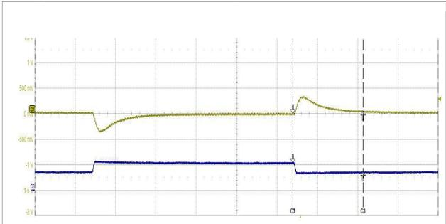
Output voltage response to load current step-
