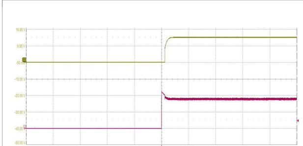
Start-up enabled by connecting  $V_i$  at:
