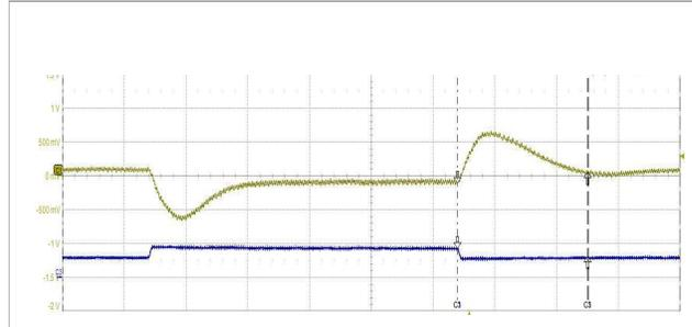
Output voltage response to load current step-
