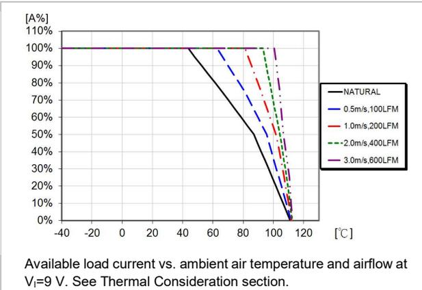
**Output Current Derating (Vin=24V)**
