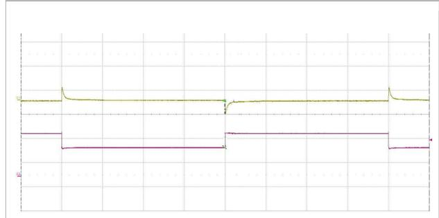
Output voltage response to load current step-
