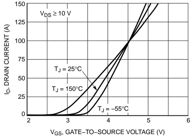
Figure 2. Transfer Characteristics
