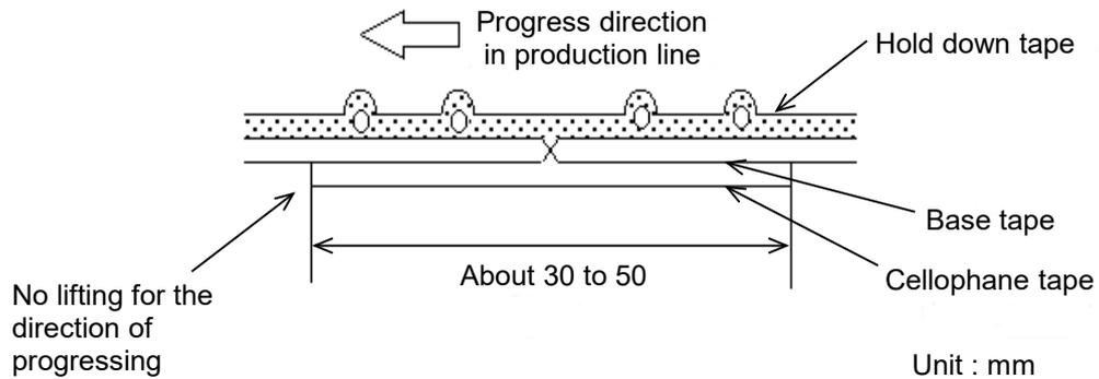
b) When hold down tape is spliced
