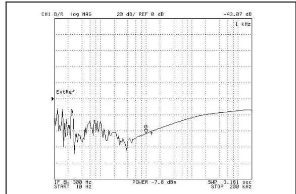
FIGURE 2-15: PSRR1-VDD (VDD = 5.0V + 0.1 V AC).
