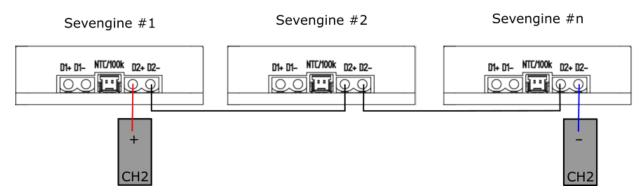
To connect the middle LED (D1+ / D1-) of the various Sevengines in series, please proceed in the same way as for the outer LEDs (CH2).
