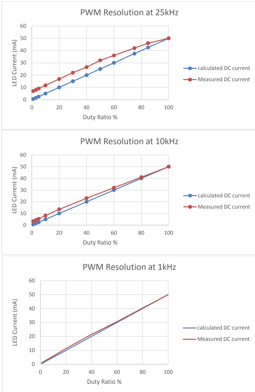
Figure 4 Typical LED Current Response vs. PWM Duty Cycle for 25kHz, 10kHz, and 1kHz PWM Frequency (See Figure 3b)
