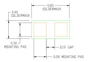
Figure 6. Recommended Mounting Pattern
