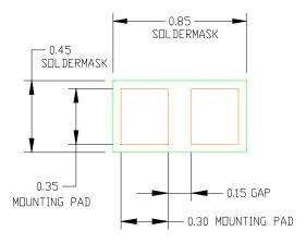
Figure 7. Maximum Recommended Mounting
