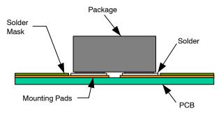
Figure 5. Cross-Section of Mounted Package
