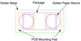
Figure 4. Recommended Mounting Pattern
