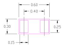
Figure 2. Dimensioned Bottom View of Package
