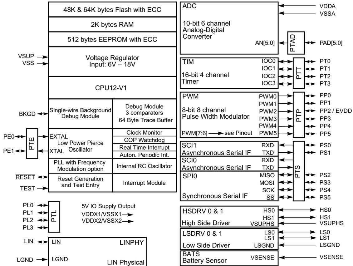
Block Diagram shows the maximum configuration!
