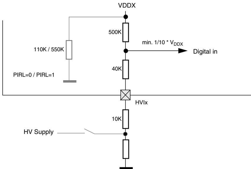
**Figure 2-48. Digital Input Read with Pullup Enabled**
