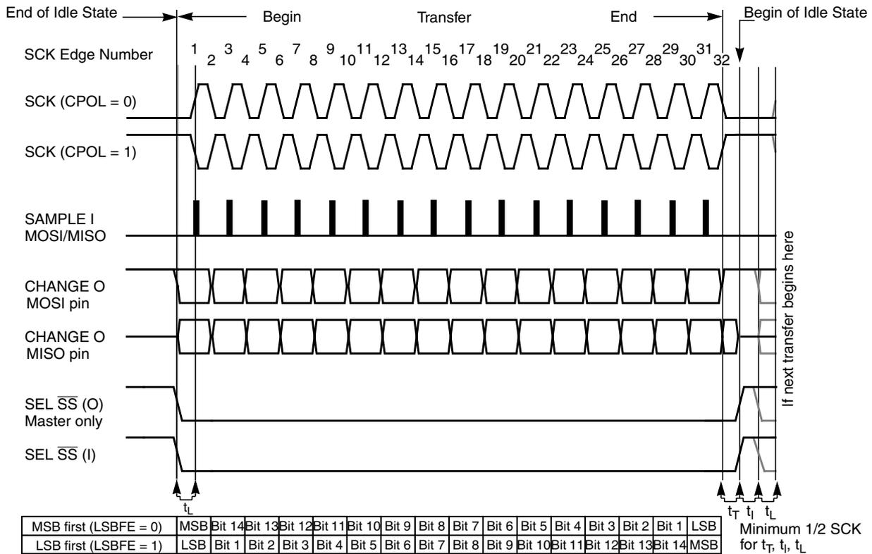
**Figure 11-13. SPI Clock Format 0 (CPHA = 0), with 16-Bit Transfer Width selected (XFRW = 1)**
