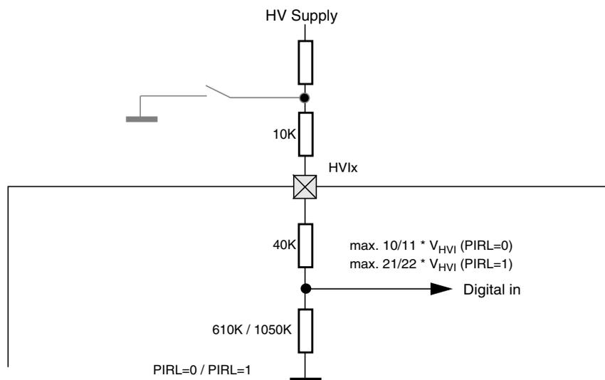
**Figure 2-49. Digital Input Read with Pulldown Enabled**
