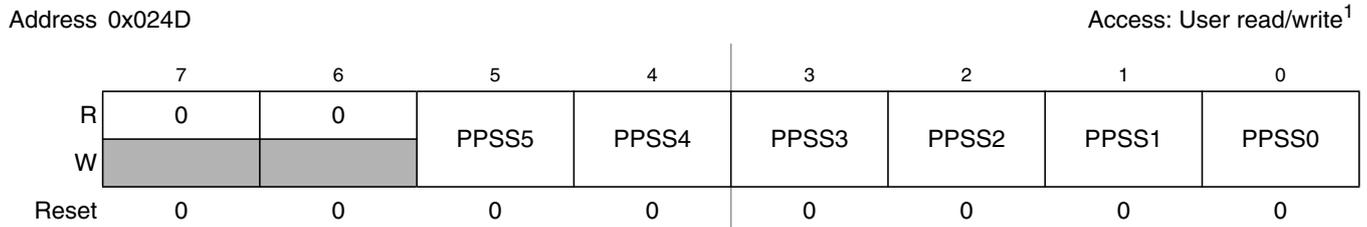
Figure 2-19. Port S Polarity Select Register (PPSS)
