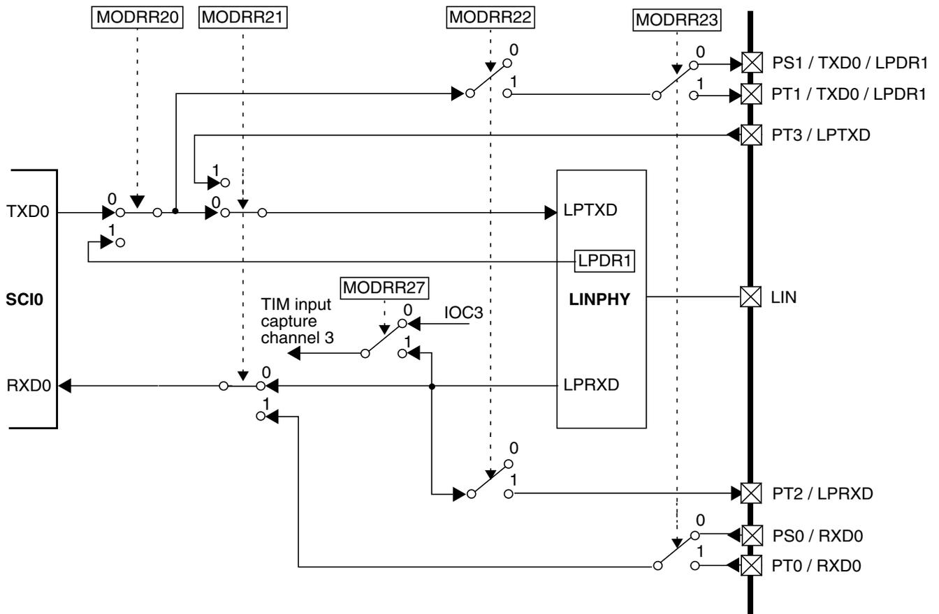
Figure 2-22. SCI0-to-LINPHY Routing Options Illustration
