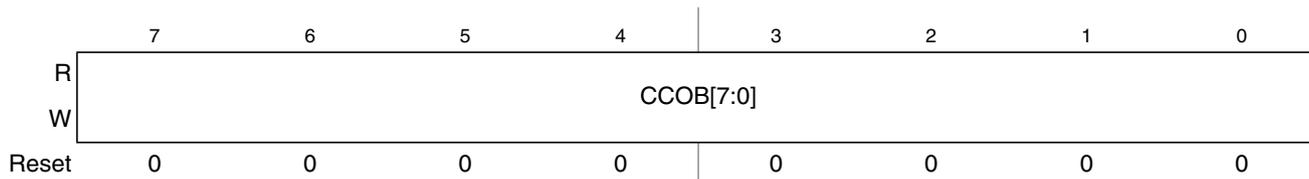
Figure 17-16. Flash Common Command Object Low Register (FCCOBLO)
