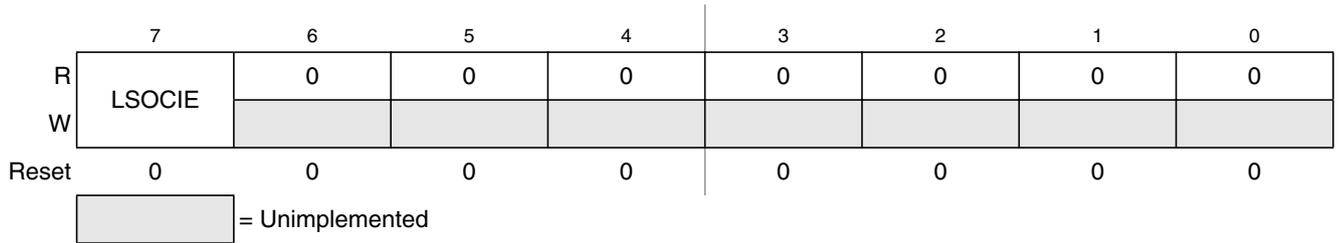
**Figure 14-5. LSDRV Interrupt Enable Register (LSIE)**
