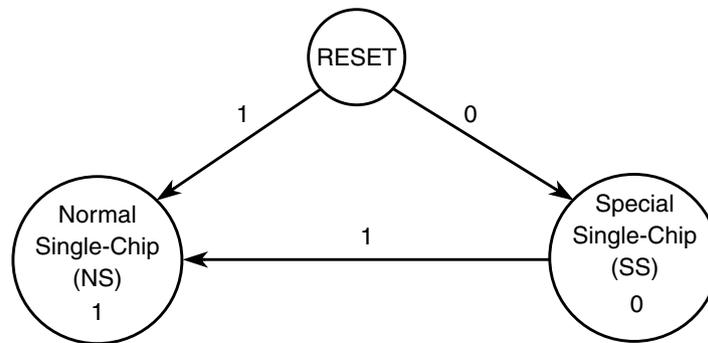
**Figure 3-4. Mode Transition Diagram when MCU is Unsecured**
