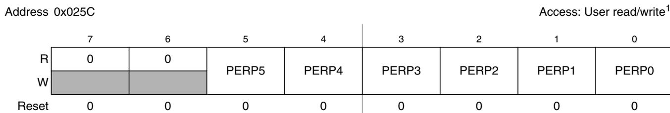
Figure 2-27. Port P Pull Device Enable Register (PERP)
