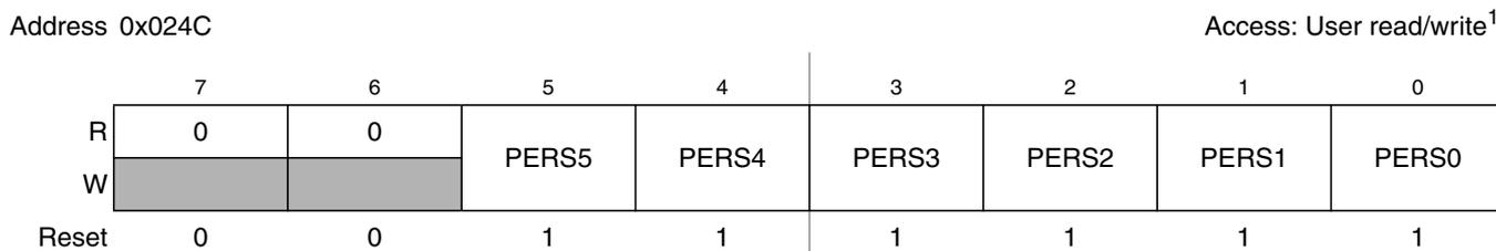
**Figure 2-18. Port S Pull Device Enable Register (PERS)**
