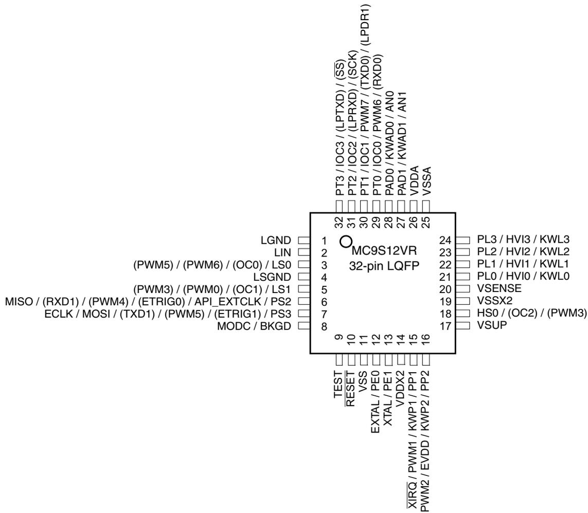
Figure 1-4. MC9S12VR 32-pin LQFP pinout
