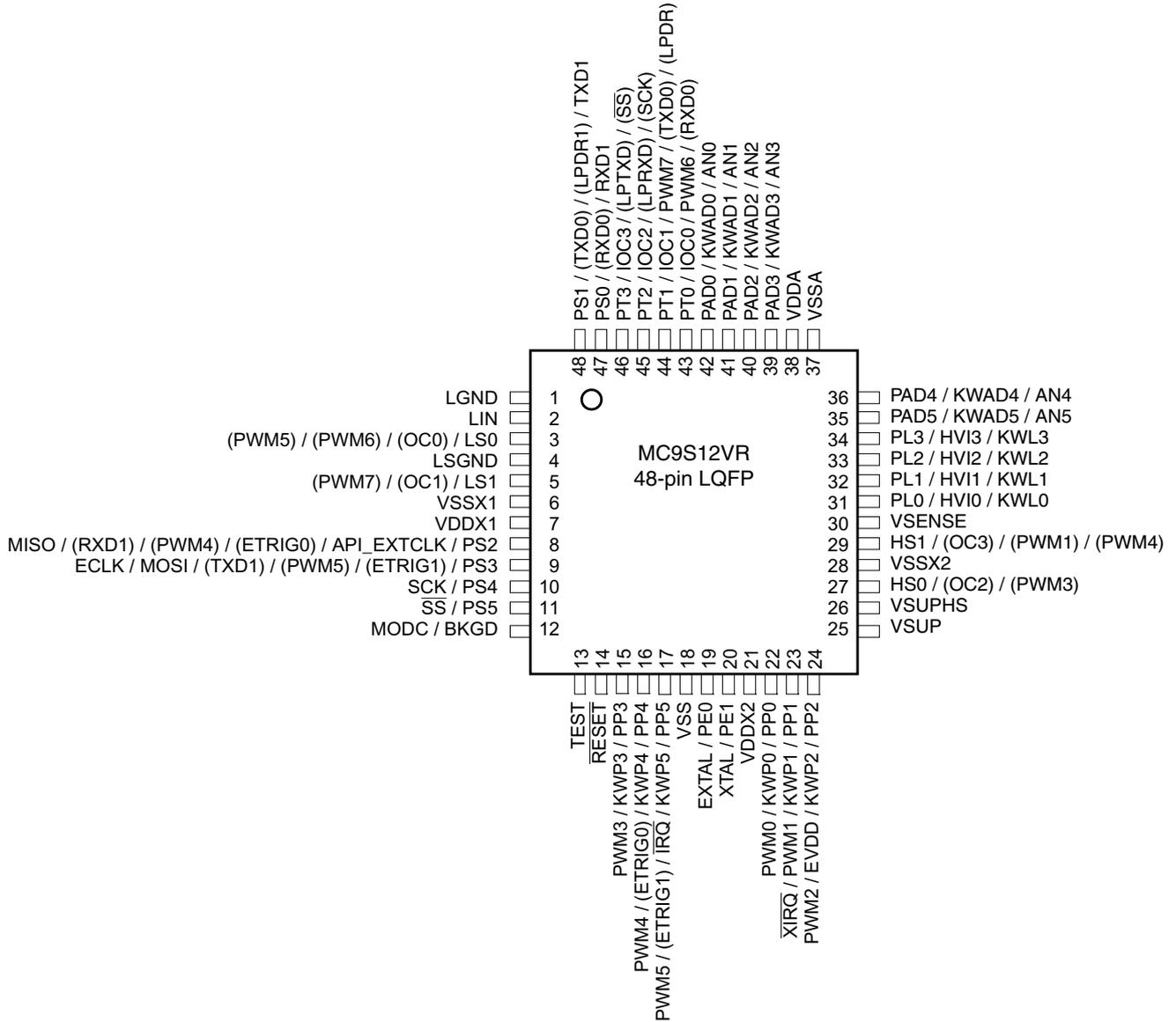
Figure 1-3. MC9S12VR 48-pin LQFP pinout
