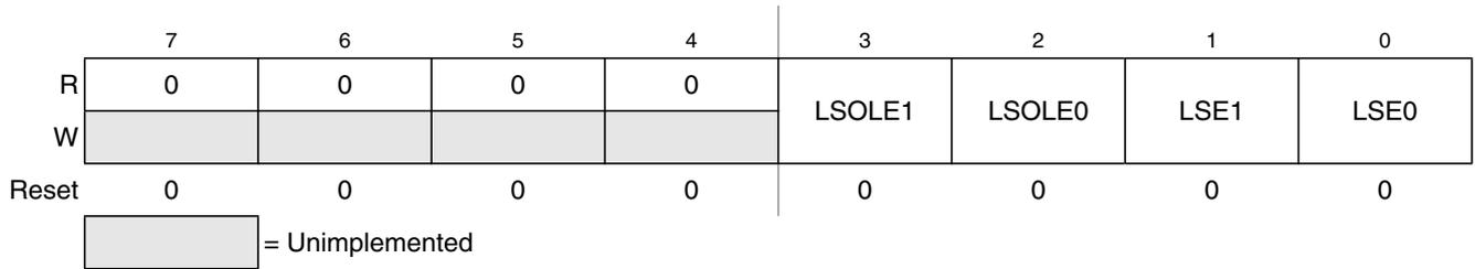
**Figure 14-3. LSDRV Configuration Register (LSCR)**
