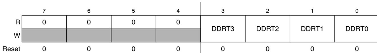
**Figure 2-10. Port T Data Direction Register (DDRT)**
