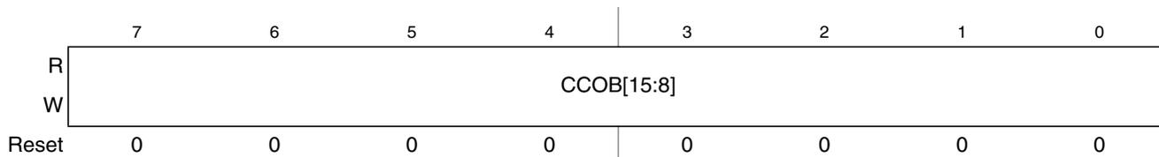
Figure 17-15. Flash Common Command Object High Register (FCCOBHI)
