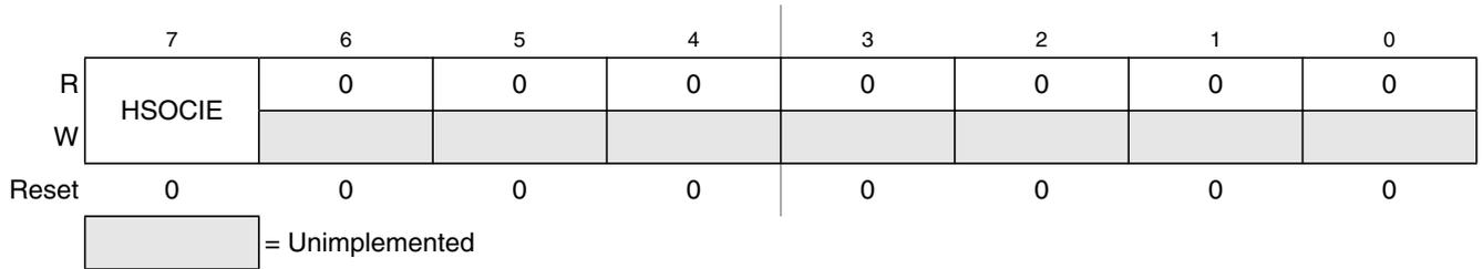
**Figure 13-5. HSDRV Interrupt Enable Register (HSIE)**
