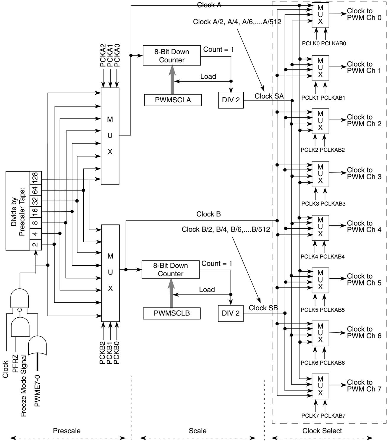
Figure 9-15. PWM Clock Select Block Diagram
