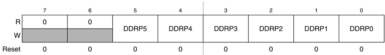
Figure 2-25. Port P Data Direction Register (DDRP)
