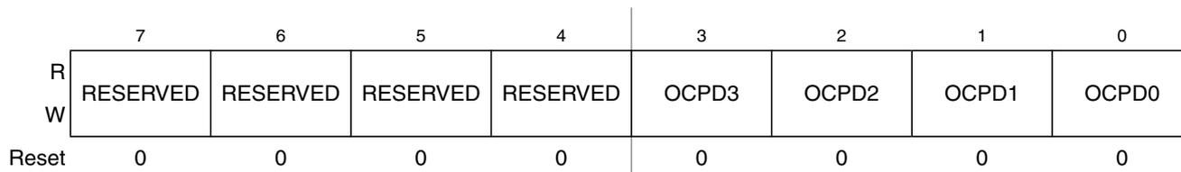
Figure 12-20. Output Compare Pin Disconnect Register (OCPD)
