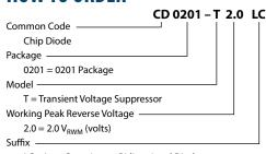
LC = Low Capacitance Bidirectional Diode
