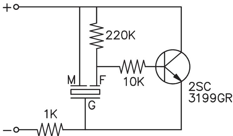
Notes: 1. The current consumption and the sound pressure level are measured by using the recommended driving circuit shown above.
