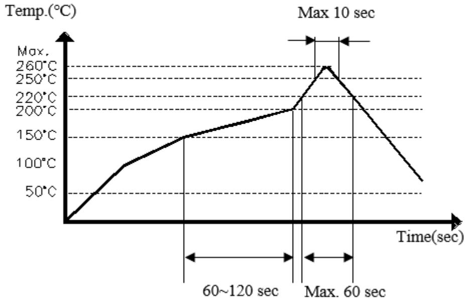
\* Reflow profile of lead-free solder
