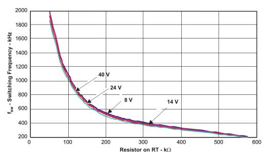
Figure 14. Switching Frequency vs Resistor Value
