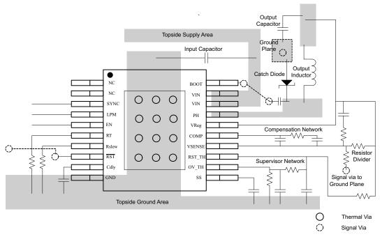
Figure 19. PCB Layout Example
