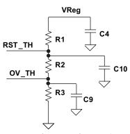
Typical cap values for RST\_TH/OV\_TH caps are between 10 pf to 100 pf range for total resistance on RSTH/OVTH divider of < 200 k $\Omega$ .
