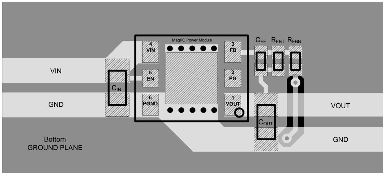
The picture above shows a possible layout for the 171010501 MagI<sup>3</sup>C MicroModule. Nevertheless, some recommendations should be followed when designing the layout:
