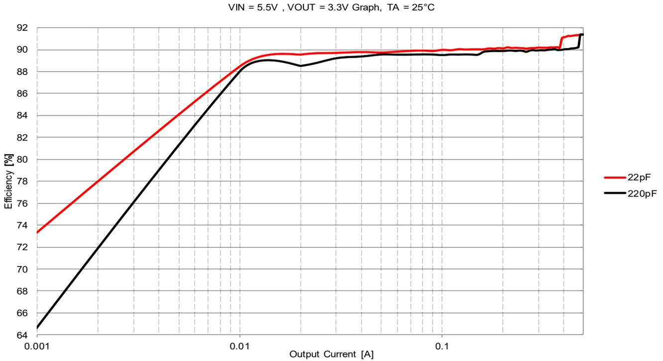
While the recommended  $C_{FF}$  value of 22pF will work for most applications, the user can adjust the performance of the MicroModule based on their application by trading between light load efficiency and transient response. This customization tailors the behavior of the MicroModule to the application's needs.
