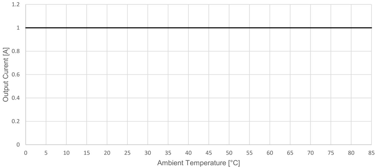
THERMAL DERATING 3.6V<sub>in</sub>171010501 Current Thermal Derating  $V_{IN} = 3.6V$ ,  $V_{OUT} = 1.8V$ ,  $\theta_{JA} = 150K/W$
