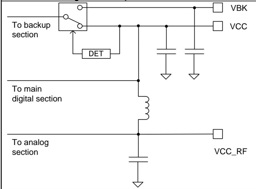
**Figure 10-3. Equivalent circuit 3**
