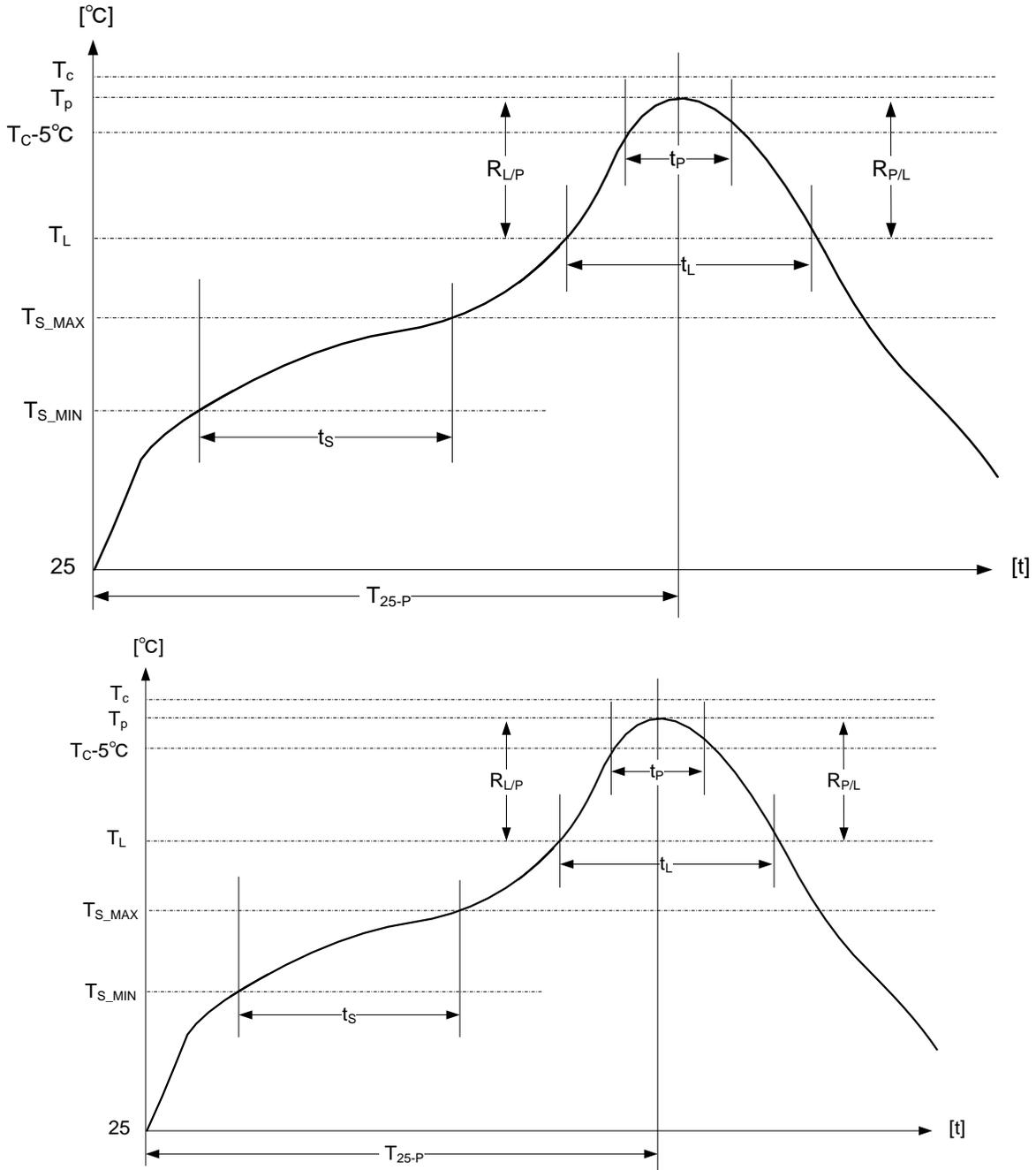
**Figure 16-1. Reflow condition**
