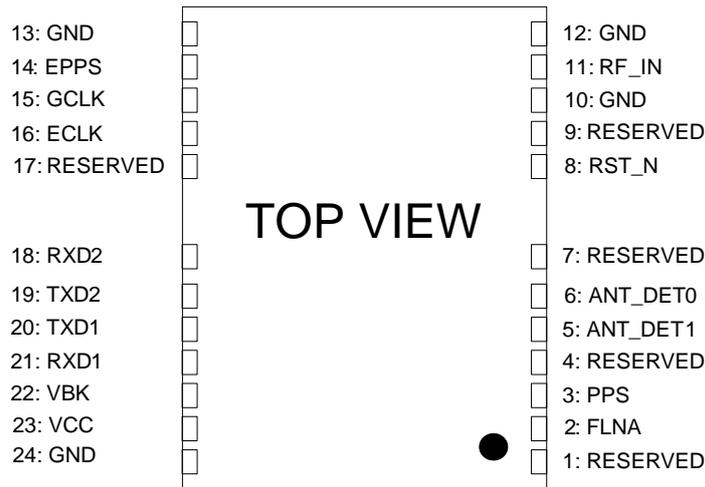
**Figure 7-1. Pin arrangement**
