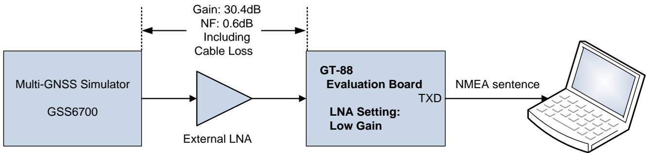
**Figure 3-1. Measurement Platform**
