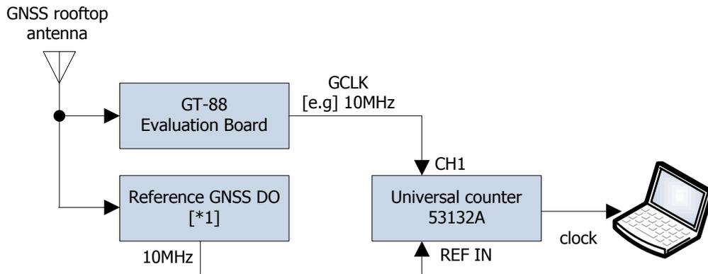
**Figure 4-2. GCLK measurement environment**
