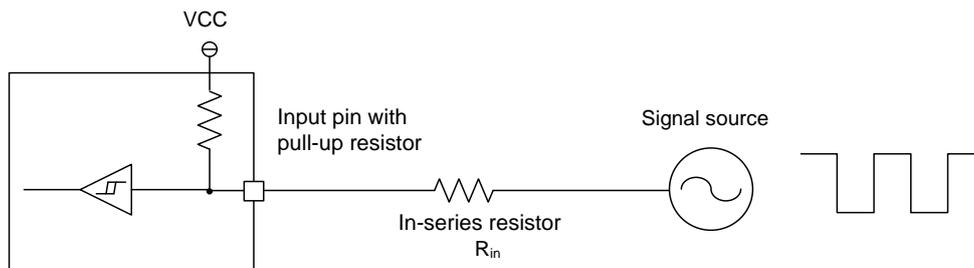
**Figure 7-2. Precaution on using the input pin with pull-up resistor**
