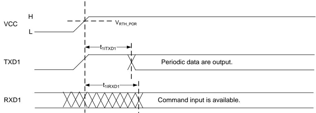
**Figure 9.6-1. UART Wake-up Timing after  $V_{RTH\_POR}$**
