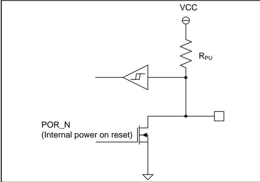
**Figure 10-2. Equivalent circuit 2**
