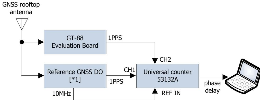
**Figure 4-1. 1PPS measurement environment**
