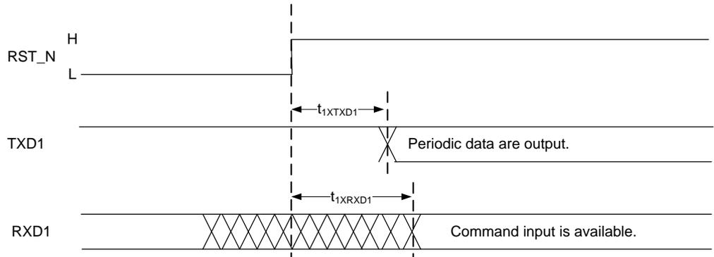
**Figure 9.6-2. UART Wake-up Timing after RST\_N**
