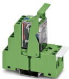
Preassembled relay modules with screw connection, consisting of: relay base, industrial relay with integrated LED and engage/disengage manual actuate lever, varistor module, and retaining bracket. Input voltage: 24 V AC, four PDTs with gold-plated contacts, 5 A
