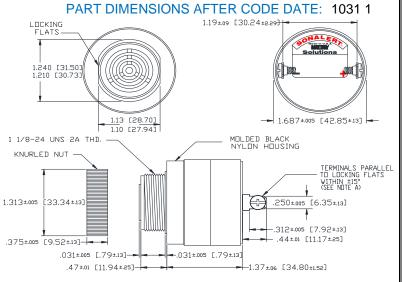
NOTE A: TERMINALS-.032 BRASS TIN PLATED, TAPPED FOR #6-32 SCREW. TVOI #6-32 NICKEL PLATED BRASS SCREWS INCLUDED. WILL ACCEPT 1/4' QUICK CONNECT.
