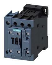
Power contactor, AC-3 25 A, 11 kW / 400 V 2 NO + 2 NC 24 V DC 4-pole size S0 screw terminals 1 NO + 1 NC integrated Traction contactor, integrated varistor
