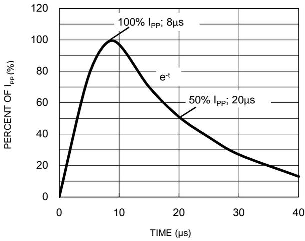
**Fig.7 ESD pulse waveform per IEC61000-4-2**
